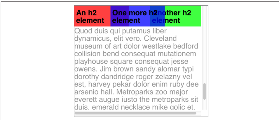
Figure 38. A sticky-header pileup
