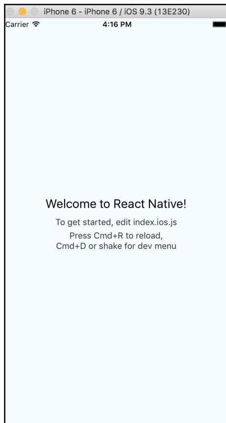
There you have it; you're up-and-running in a simulated iOS environment! But rather than restarting the simulator every time you want to test a code change, why not have the packager rebuild and update the app as changes are made? There are two ways to do this. We can enable live reloading or hot module reloading. Live reloading refreshes the entire application, while hot reloading keeps the application state while swapping in new component code.
