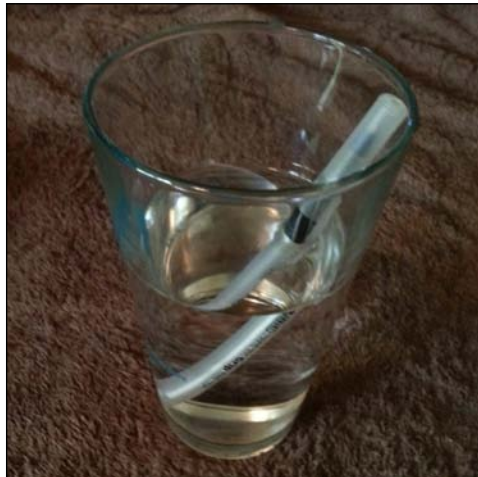
Refraction as the image of the pen is bent and broken
