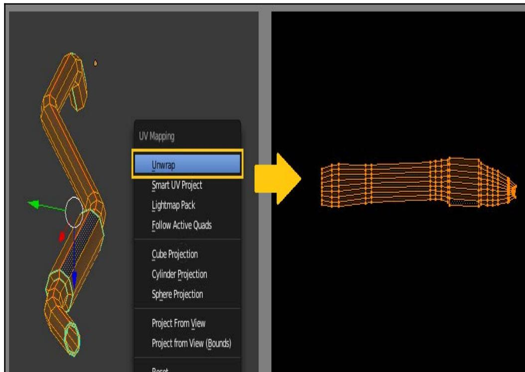
The resulting UV map may look a bit strange, but it does make sense when you think about it. Because the different parts of the exhaust have different diameters, the UVs will have be a little taller/wider in some places to make up for that.
