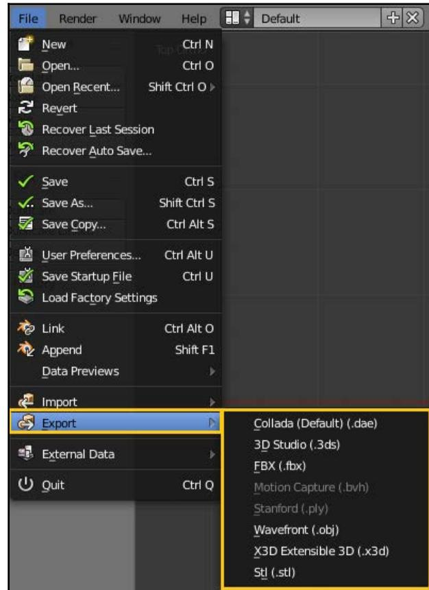
These are the formats that Blender can directly export to (and there are more that can be activated with add-ons). Additionally, there are other methods (some online) that can be used to convert one model format to another. Many game and simulation platforms also have import functions, allowing you to bring in a model from another format.
