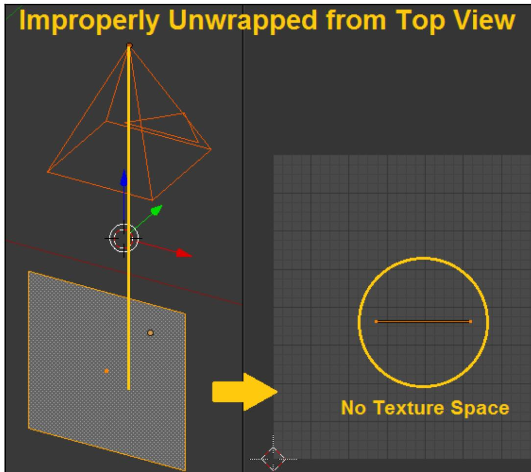
To avoid that problem, you can unwrap the model from almost the bottom view. If you unwrap it, say, 15 degrees off the axis, you should get an adequate result:
