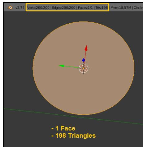
Sure, there's only one polygon being displayed, but you're using 198 triangles. What this means is that your mesh isn't nearly as efficient (or "low-poly") as you thought it was.
