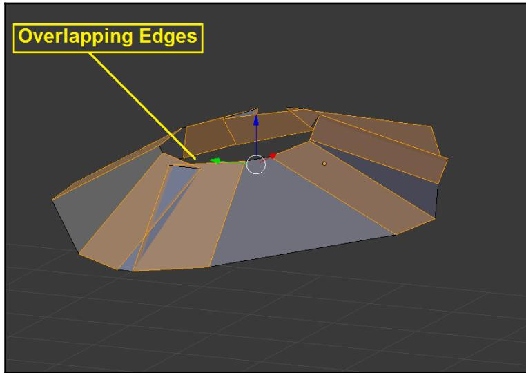
That's kind of a mess, isn't it? This type of overlap tends to occur when the vertices are closer together at one end than at the other:
