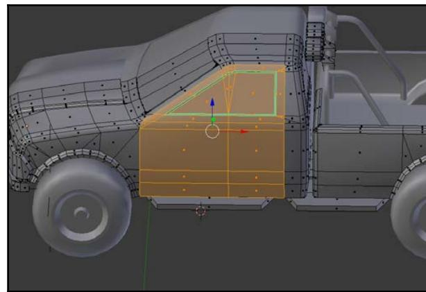
Using the **Inset** tool, we can create a slight panel line where the door connects to the body. This is another case where we don't technically need to do that (it uses polygons), but there may be a benefit.
