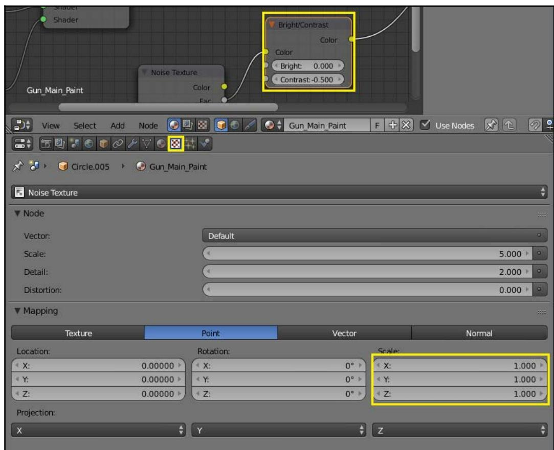
You can also adjust the overall scale of the texture. This is done directly in the **Noise Texture** node. By changing it, you can make the texture appear larger or smaller. You can adjust this as needed until you get the desired effect.
