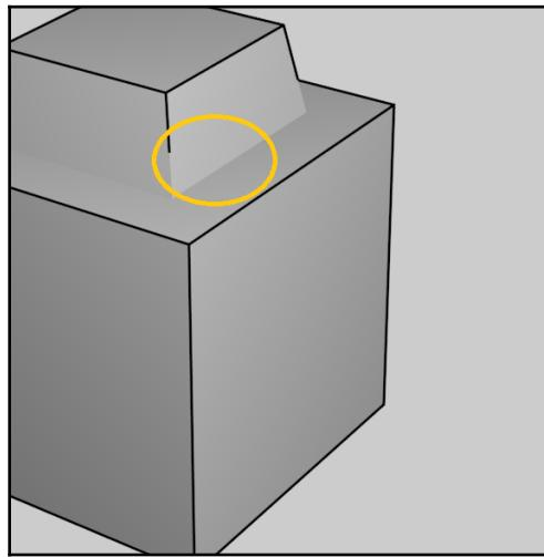
One solution is to connect all the vertices in a mesh, creating *watertight* or *non-manifold* geometry:
