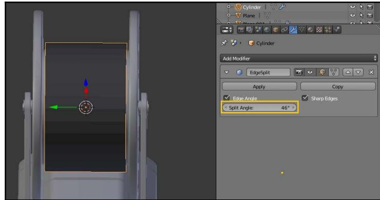
That way, edges that would normally be sharp (more than 30 degrees) will be smooth. The reason for this is just that we're going to add a lot of geometry to the reel anyway (the cable is very thin), and I don't want to have to bevel it a huge number of times:
