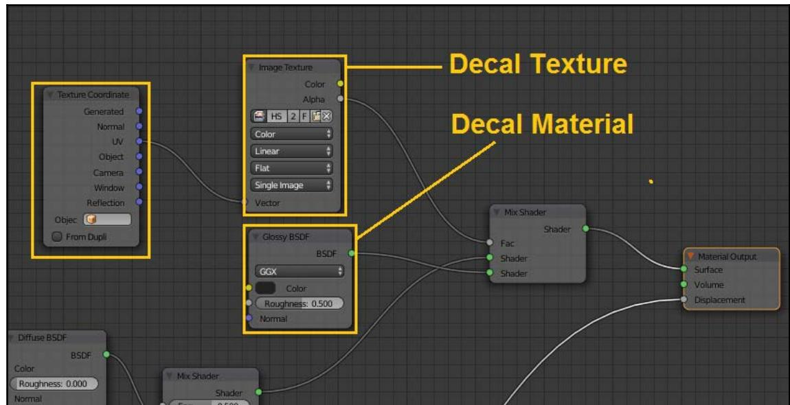
You can see here that I'm using a **Texture Coordinate** node (found under the **Input** submenu). This tells Blender to use the UV coordinates to align the image.
