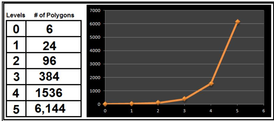
In practice, it would be rare to add more than two or three levels of Subdivision Surfacing. Still, the polygon count is one of the main drawbacks to it. **Subsurf** is a quick way to get smooth, flowing shapes—but, at a cost.
