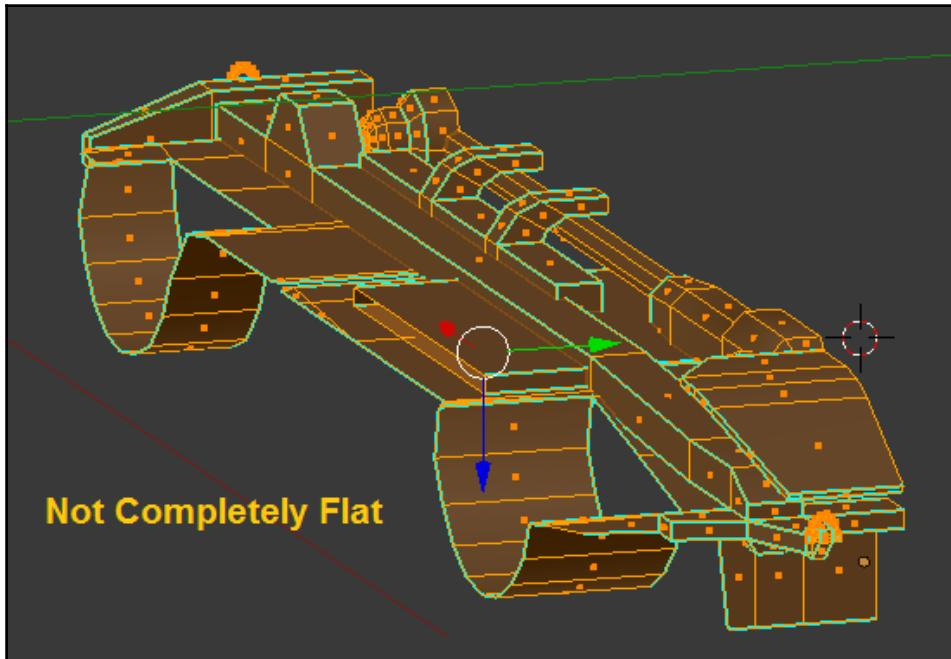
You can see that bottom of the truck is *almost* flat. In other words, it looks like it could mostly be unwrapped from the bottom view. That's very tempting, as it would save a lot of work. However, you can see that there are a few little parts that would need to be unwrapped from the side view.
