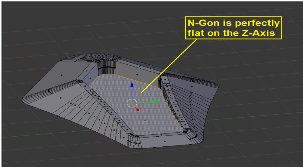
Before we go further, let's duplicate the upper section and flip it down across the Z axis (using *Ctrl + M*):
