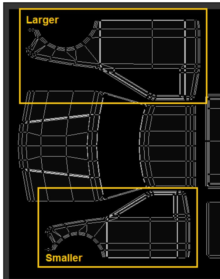
One way to fix this is to add a new image in our **UV/Image Editor**. Under the **Generated Type** option, we'll pick **UV Grid**:
