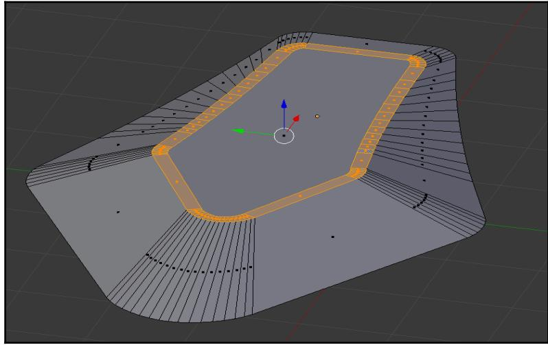
Then, we'll extrude that N-Gon down slightly into the hull and scale it to zero on the Z axis (S, Z, 0):
