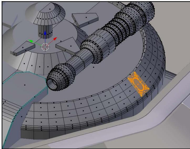
You can then set your **3D Cursor** to the center of that circle and rotate the cutout piece into position (you'll have to delete the original geometry first). Once you do that, of course, you'll need to remove the doubles you created. This saves you the trouble of cutting all those shapes in one at a time:
