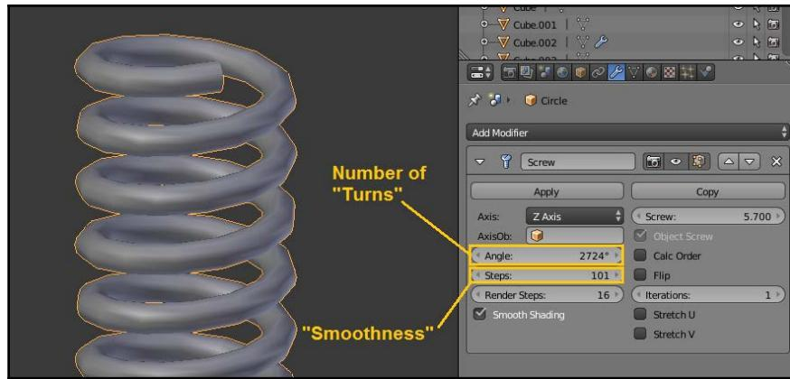
Go ahead and play with these until you're happy, then move and scale your spring into position. Once it's the way you like it, go ahead and apply the **Screw** modifier (but don't join it to the shock absorber just yet):
