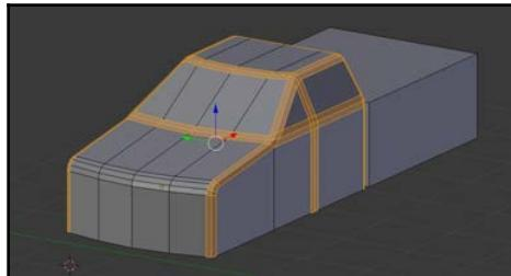
Next, I'll add an edge split modifier to the mesh. We'll use a split angle of 47 degrees or so. I wanted to make sure all the 45 degree angles were smooth, so I just added a couple of extra degrees in case there was a weird corner in the mesh somewhere.
