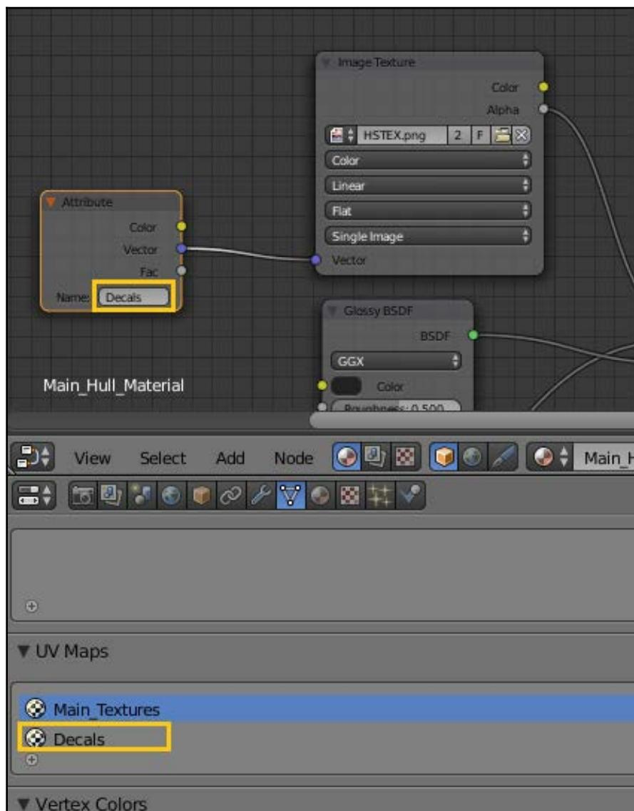
One problem you may run into when doing decals is that UV maps (just like the mesh itself) are mirrored between the two sides. This means that if you unwrap some words or letters on one side, they will be “flipped” (mirrored) on the other side.
