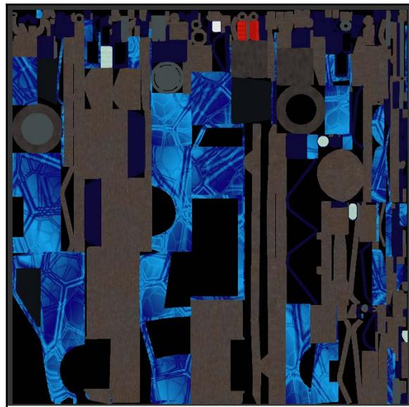
However, we do have a slight problem with the way we baked it. Because we used a mirror modifier on the model, Blender tried to bake both sides of the truck to the same 2D texture space. However, the paint pattern is not symmetrical (it's different from one side to another). There's no way to bake both halves of the truck to the same 2D space.
