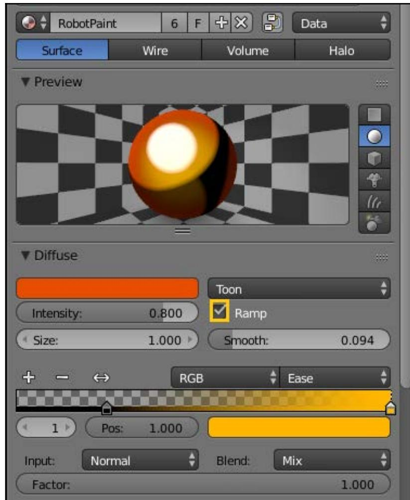
It can be used to simulate color changing paint, glass, or anything else where the color varies with the angle. The setup shown is pretty basic, but I think it makes the robot look a little bit better:
