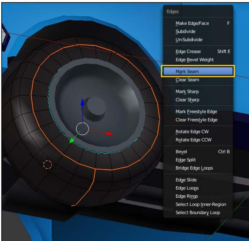
I've marked a seam here as well. Since we'll want to draw a tread pattern onto our image later, we need to make sure that the tire is unwrapped appropriately. Also, unwrapping the sidewall portion from the side view will give you the opportunity to add a bit of text or other details to the side of the tire:
