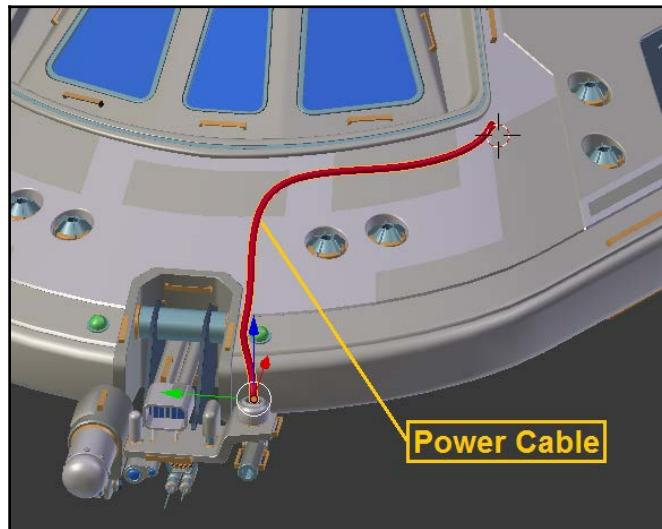
By the way, you don't need to add multiple **Path** objects to your scene (generally). Within **Edit Mode**, you can copy an existing **Path** and just move it to a new position. That way, any changes you make to its characteristics (diameter, resolution, and so on) will apply to all of your Path objects. If you want to change the diameter of just one or two sections, you can use *Alt + S* to adjust their diameter in **Edit Mode**:
