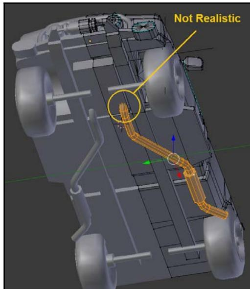
This can be frustrating when you build game models. Cars are a hobby of mine in real life, so I know that the exhaust pipes should run into a header (or exhaust manifold), which in turn should connect to the engine block. My natural instinct is to do that with the model. However, that would probably be a mistake. We'd be adding a lot of geometry to an area of the truck that's rarely seen.
