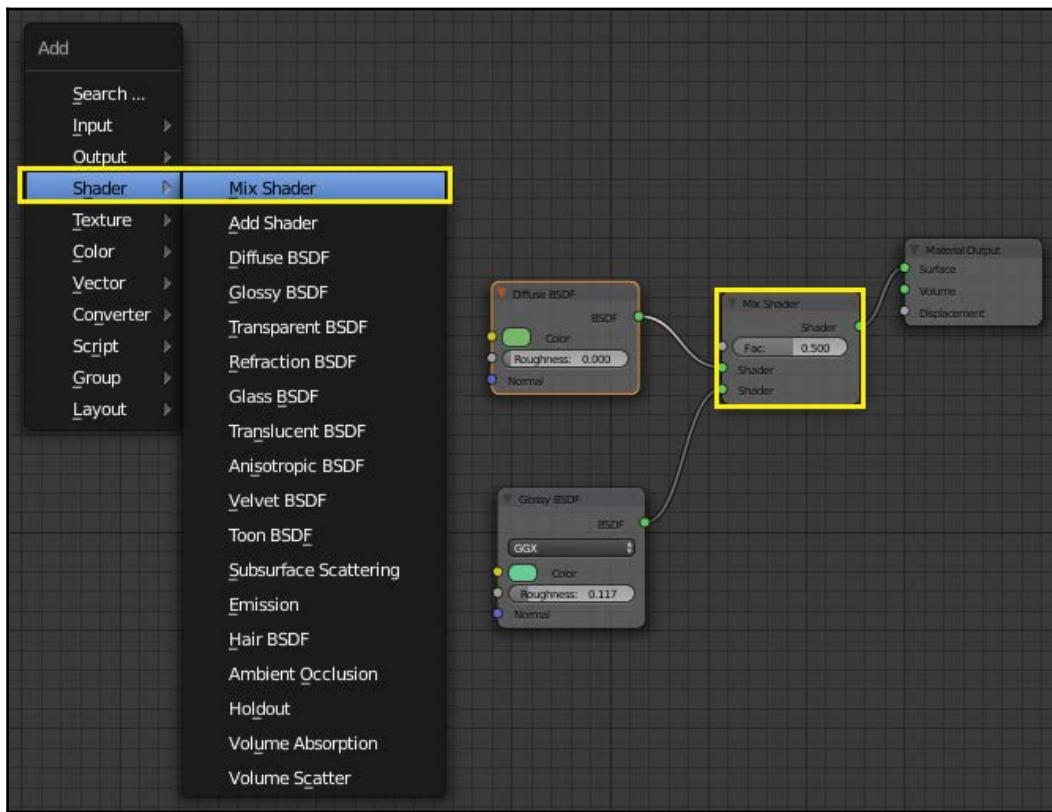
Connect the outputs of both the **Glossy** and **Diffuse** shaders to the **Mix Shader**. Then, connect the **Mix Shader** output to the **Surface Slot** of the **Material Output**.
