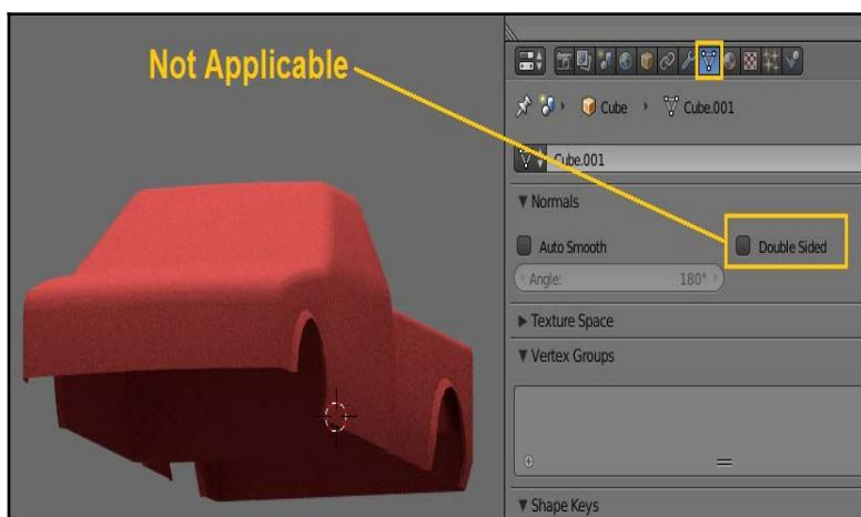
To make sure we don't have any problems with the back side of polygons, the best solution is to fill in the geometry so that we have no open or "non-manifold" meshes.
