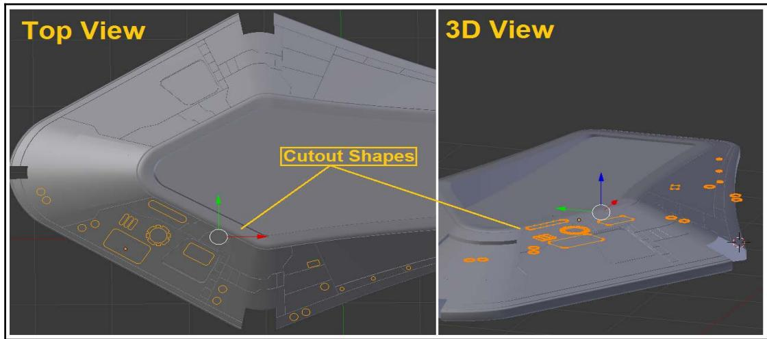
Using the same techniques from Chapter 2, *Sci Fi Pistol – Adding Details*, we'll cut those pieces into our hull:
