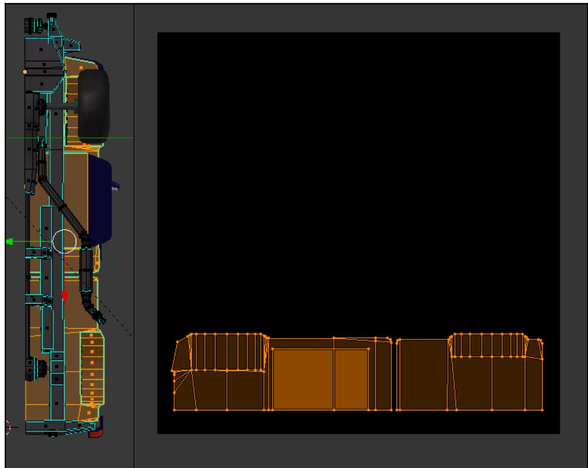
Next, we'll unwrap the exhaust pipe. You can do this by selecting one of the long edge loops along the pipe and marking a seam. A seam tells Blender where to cut the model in order to unwrap it. By specifying which edges are going to be seams, you gain a lot more control over the unwrapping process. In order to mark a seam, you simply hit *Ctrl + E* and select **Mark Seam**:
