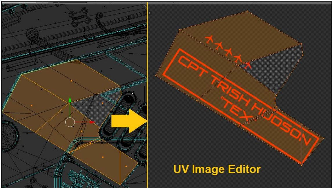
You can assign multiple parts of the model to the same area of an image. If a decal is repeated, it's easy to use one image and replicate it.
