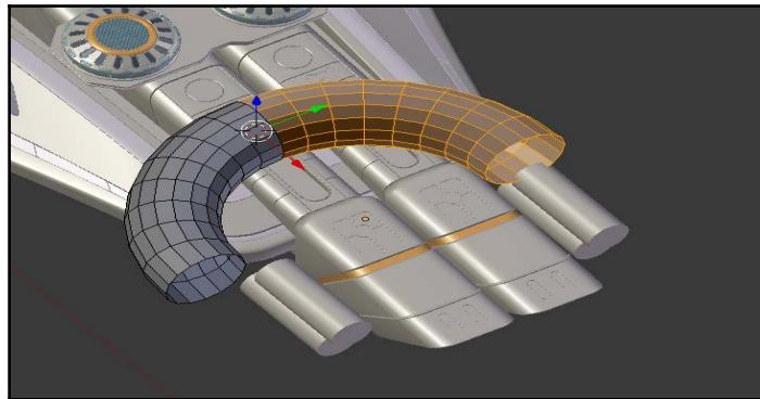
Then, I can rotate one side by 90 degrees around the **3D Cursor**, giving me a nice bend to my pipe:
