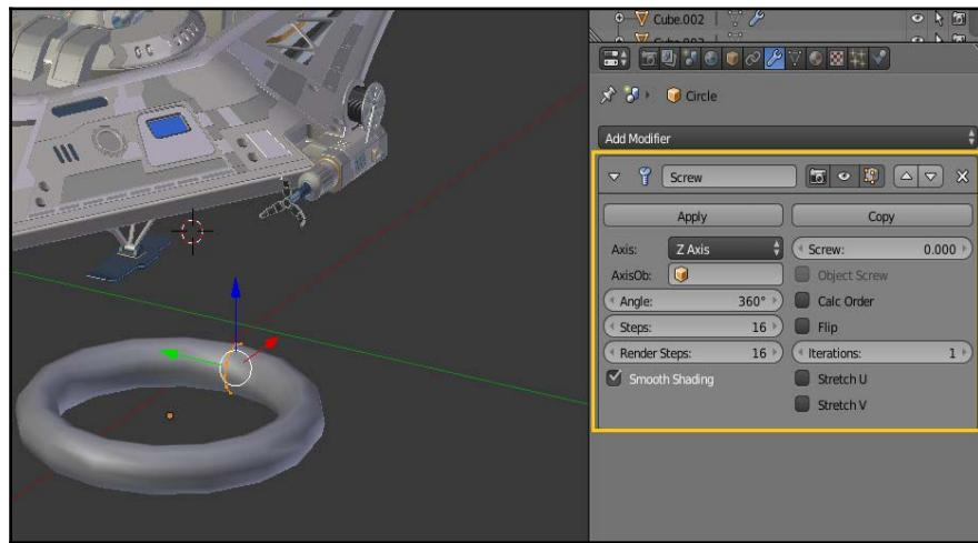
There are a couple of settings you'll want to make note of here. The **Screw** value controls the vertical gap or distance of your spring:
