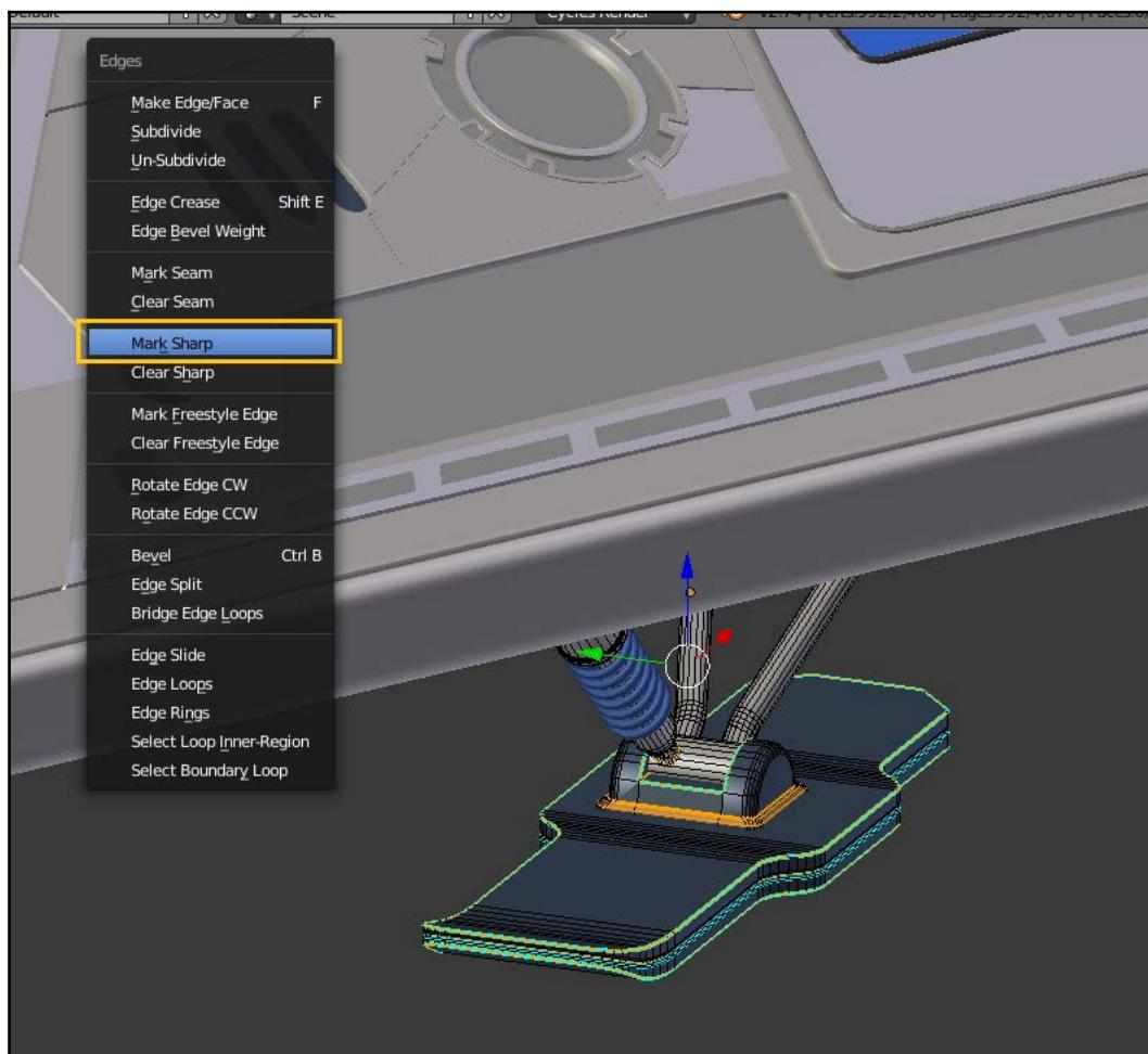
Since all the 30 degrees angles are marked sharp, we no longer need the **Edge Angle** option on our **Edge Split** modifier. You can disable it (unchecked it) and the landing gear remains exactly the same:
