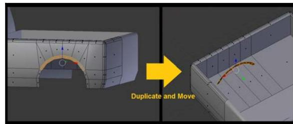
Then, we can delete the faces we don't need and build that wheel well into the mesh of the bed.
