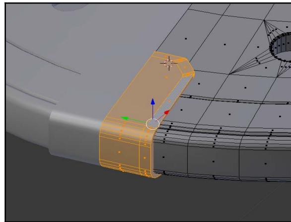
We can then delete the faces created inside the loop and bridge the top and bottom edge loops to create our final shape:
