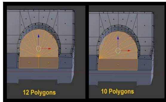
This tends to look a bit messy, though, and can sometimes make it difficult to see how meshes are put together. You'll have to decide how important polygon efficiency is for your application. In this case, I don't feel that saving two polygons is worth it. The final truck is around 5,000 polygons (as mentioned before), so we're talking about less than a 1% decrease in efficiency here (0.04%, actually).
