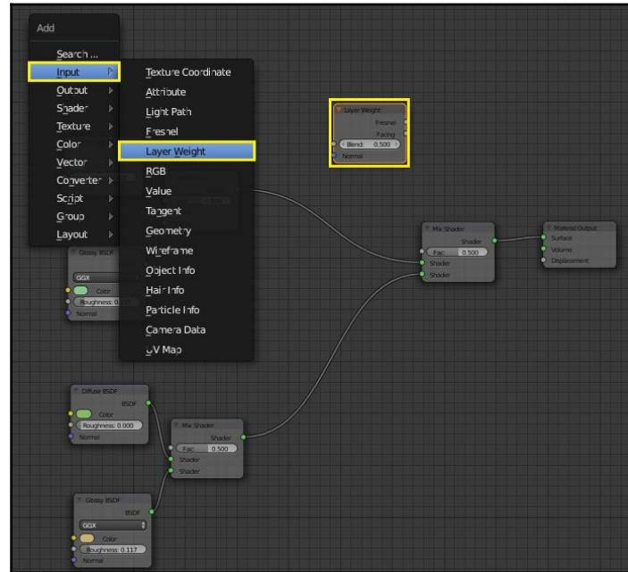
Connect the **Facing** tab of the **Layer Weight** input to the **Fac** (Factor) input of the **Mix Shader**.
