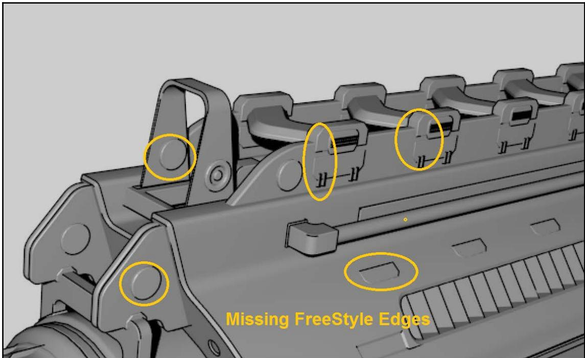
It looks like we're missing lines where the small detailed pieces join with the main body. That's because there's no actual connection there – the detailed piece is just sitting on (and slightly penetrating through) the main mesh. That works fine for normal rendering, but it confuses Blender's Freestyle function.
