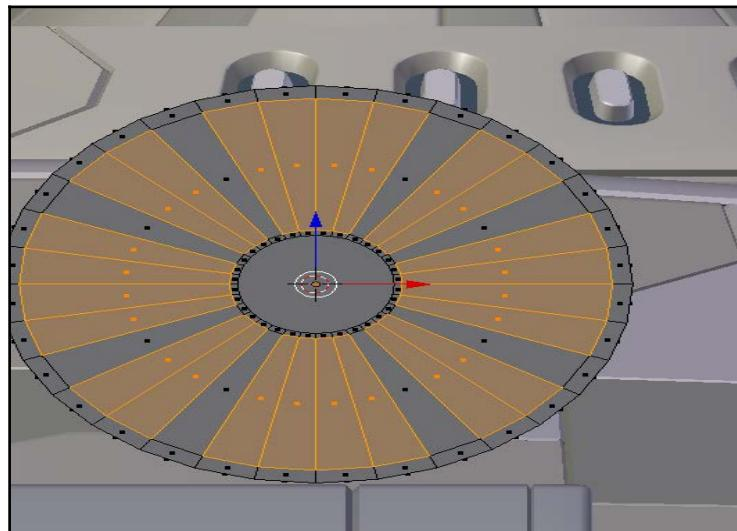
Then, we can round out those corners and add struts to connect it to the main section of the grappling gun:
