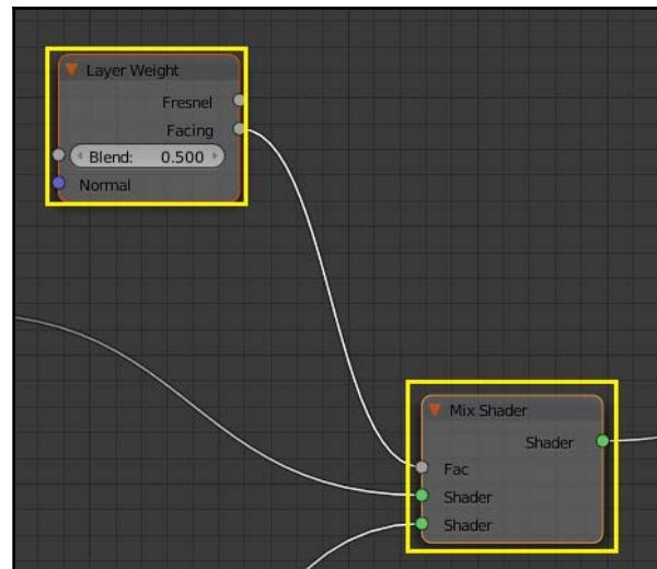
Since we're using solid (metal/ plastic) types of materials, it's best to use the **Facing** output of the Layer Weight shader. If you have a material where light penetrates the surface (such as glass or translucent plastic), you can also experiment with the Fresnel tab. For now, we'll stick with **Facing**.
