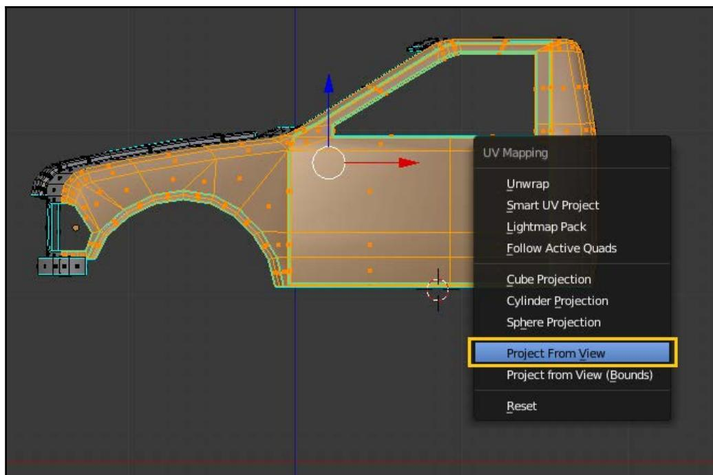
You can repeat this process for the other parts of the body and move the resulting UVs around until they form a rational pattern:
