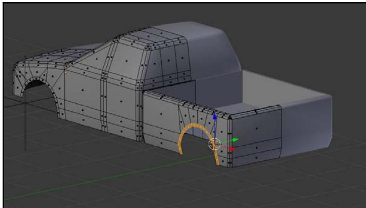
Afterwards, we'll duplicate a portion of that circle and move it in towards the center of the truck bed. This way, we can create the shape of the wheel well inside of the bed.
