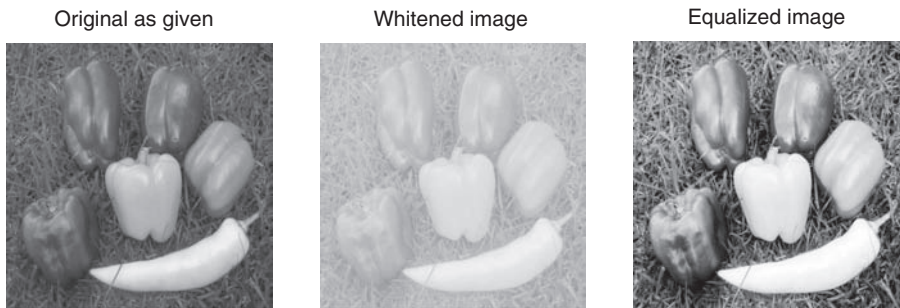
FIGURE 4.13 Illustrating histogram equalization, with the original image shown on the left. It is assumed that this image is not available. The image as presented is shown in the middle, and this is used as input to the histogram equalization algorithm. The output of the algorithm is shown on the right.
