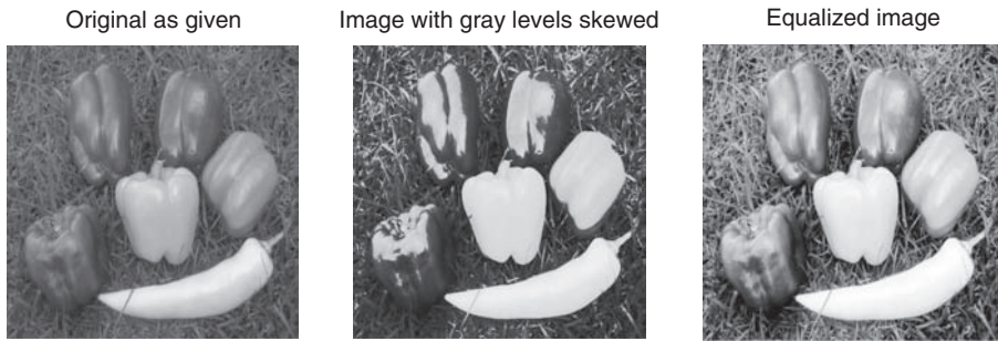
FIGURE 4.15 Histogram equalization with skews in both directions. The image histogram is moved both toward the black end of the scale for darker pixels and toward the white end for lighter pixels, resulting in the middle image. Histogram equalization applied to this image results in the image shown on the far right.
