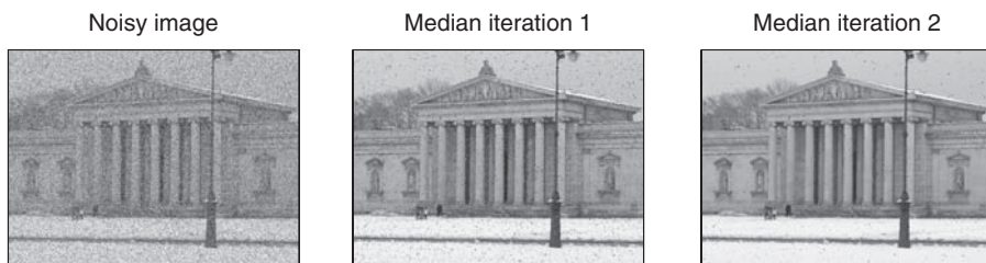
FIGURE 4.22 The effect of multiple iterations on the median filter. The noise-corrupted image is again on the far left, with the other images being the median filter restored images after one and two iterations, respectively.
