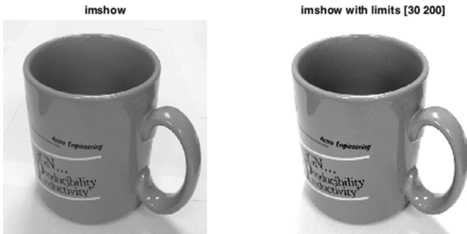
Figure 3-21. Mug displayed using imshow , with color limits applied on the right
