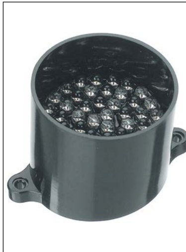
The Kingbright infra-red LED cluster runs from a 6V supply, which means you can connect two in series — one on either side of the camera.
