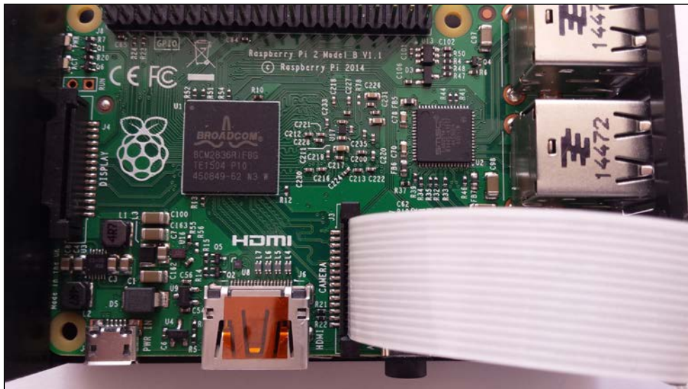
Connect the camera module to the dedicated interface
