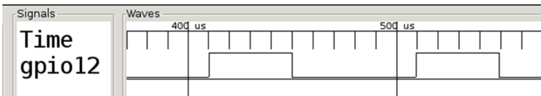
Figure 7-5. PWM 40% signal with S = 10
