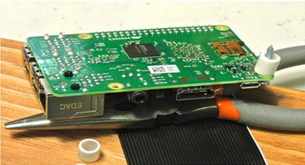
Figure 2-8. Spacer and wood screw protruding
