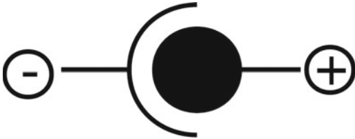
Figure 4-4. DC power adapter center positive indicator
