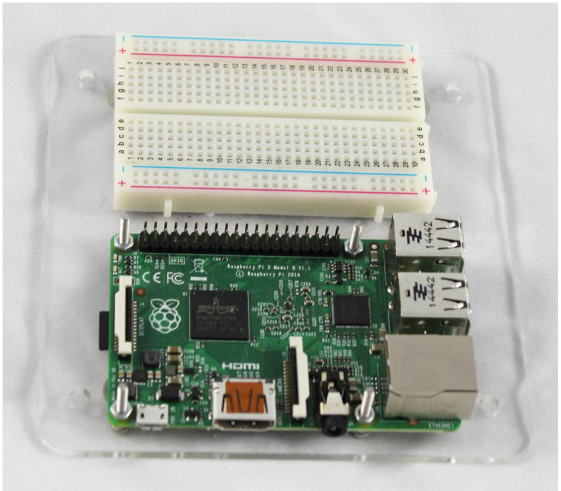
Figure 1-5. Raspberry Pi and a breadboard mounted together
