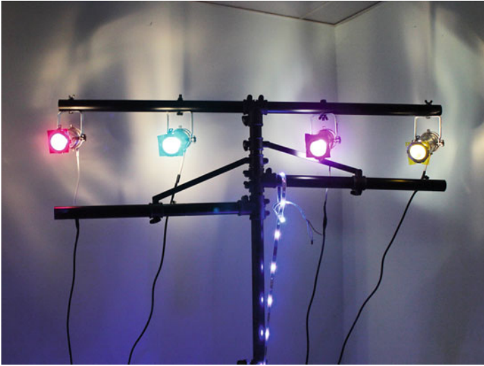
Figure 4-22. PAR 16 spotlights used as multi-colored disco lights
