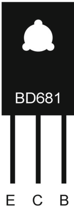
Figure 4-20. BD681 Darlington Transistor pinout
