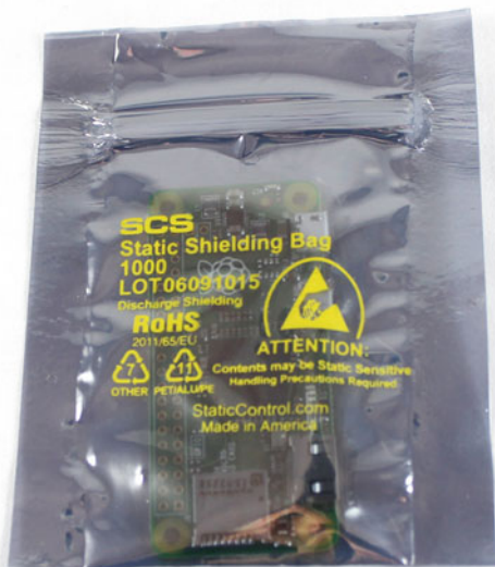
Figure 1-10. Warning symbol for a static-sensitive component
