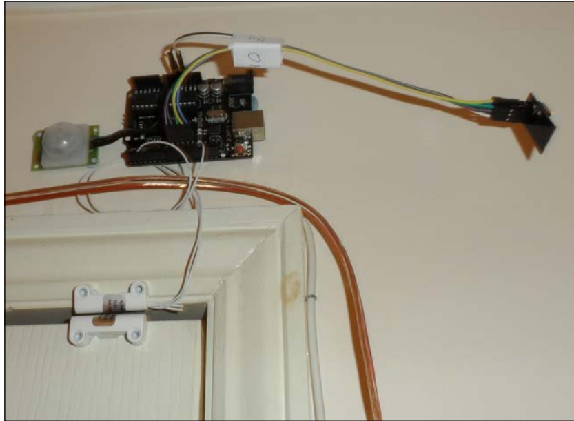
The sensor node with a door switch and PIR sensor installed above a door frame using Blu-Tack
