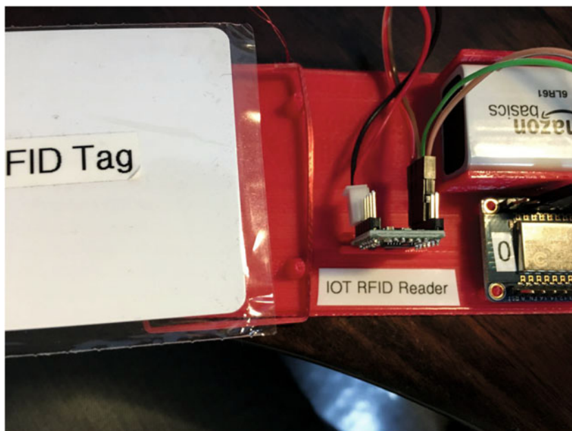
Figure 6-8. RFID Tag Card over the IOTRFID Device
