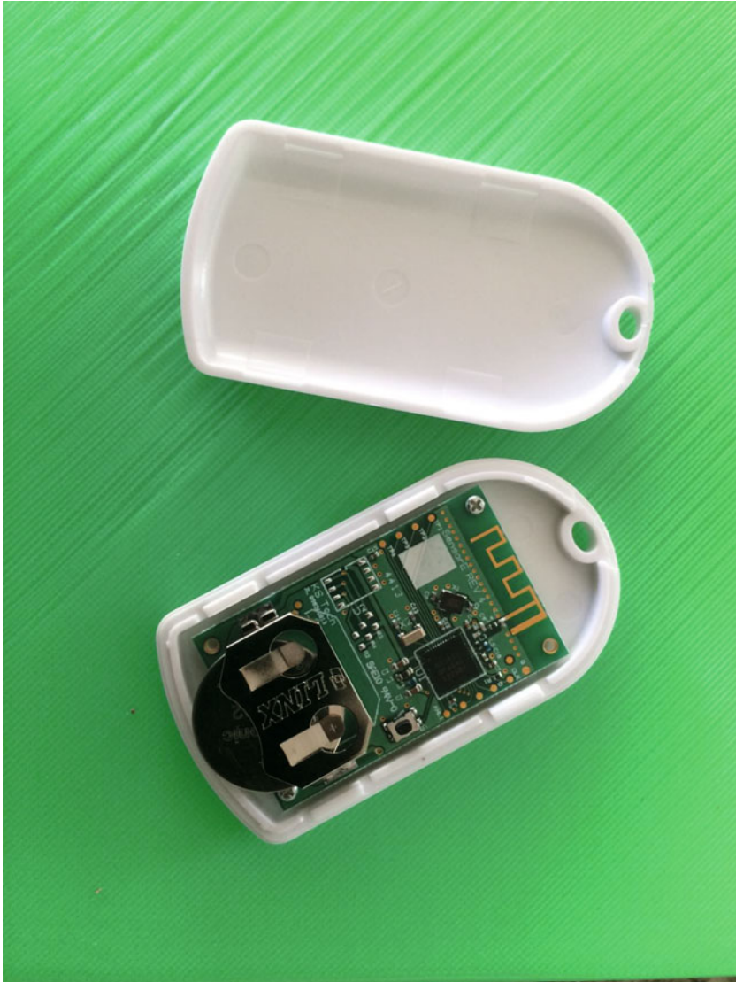
Figure 4-3. Inside of a Particle iBeacon
