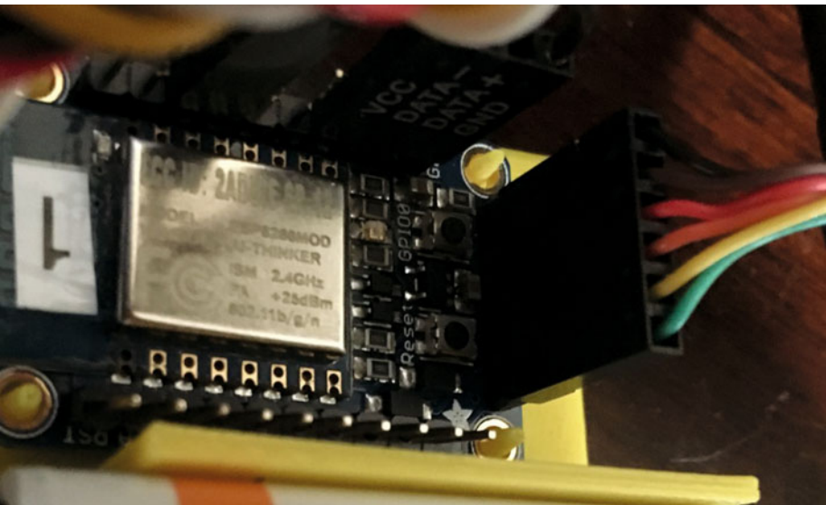
Figure 2-9. FTDI Cable Plugged into ESP8266
