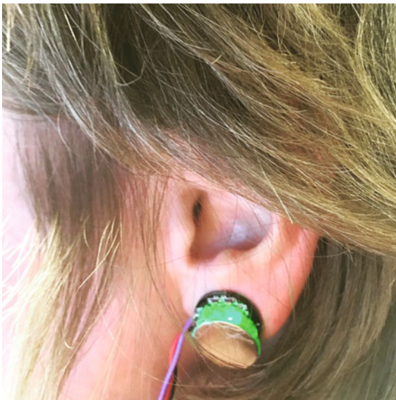
Figure 5-9. IOTPulse Sensor on Ear
