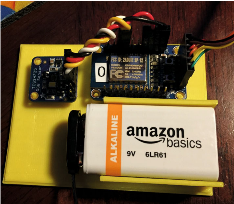
Figure 2-11. A Complete LightSwarm Device
