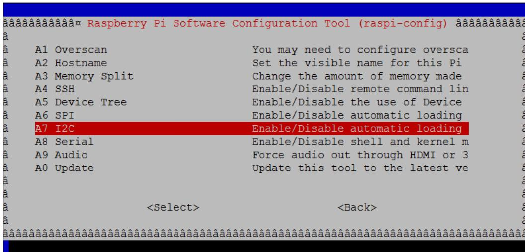
After finishing, Raspbian loads the I2C module automatically when starting up. You can verify this by checking the `/boot/config.txt` file. You should see `dtparam=i2c_arm=on`.
