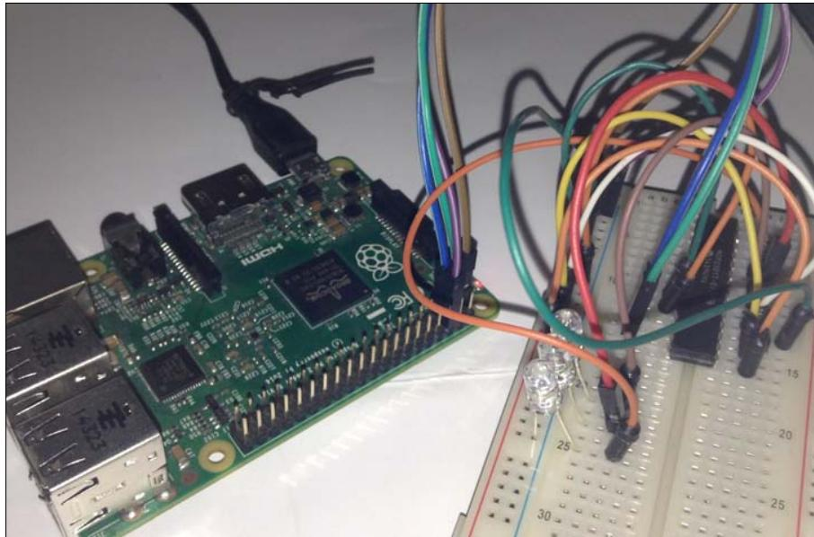
After completing the wiring, you can plug the DC adapter into Raspberry Pi to power up the board. To verify that our wiring is correct, you can use a `i2cdetect` tool, a part of I2C tools. Please read *Chapter 3, Make Your Own Digital Clock Display* to review Raspberry Pi I2C.
