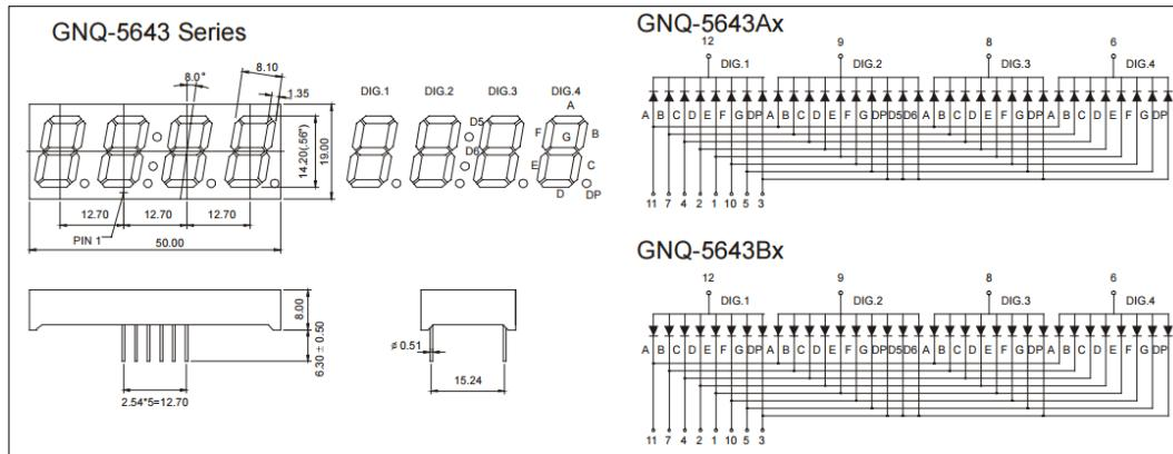
You can see that four 7-segment display modules have been connected and shared on *a, b, c, d, f, g*, and *DP* pins. To display the first digit on 7-segment, you can set a value *high* on digit-1 (DIG 1). Otherwise, you can display the second digit on 7-segment by setting a value *high* on digit-2 (DIG 2). It means only one 7-segment display is running. You can run all 7-segment displays by manipulating the delay shown on this module.
