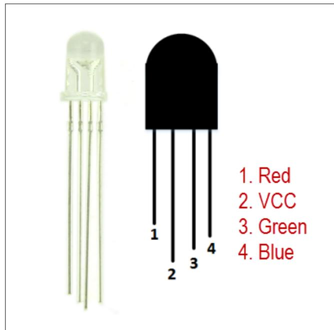
In this section, we will build a simple program to display red, green, and blue colors through the RGB LED.
