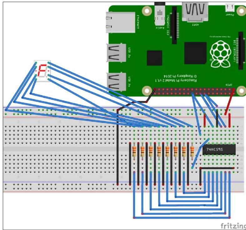
You can see that there are resistors on the wiring. These components are used to prevent the higher current flow on your wiring so a resistor keeps your IC module safe. You can ignore these components if you can guarantee the safe current flow on the circuit.
