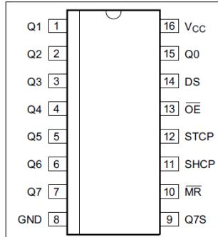
The *Q0* to *Q7* pins are the parallel output from the chip. The *DS* pin is the serial data. *STCP* is the latch pin, and *SHCP* is the clock pin.
