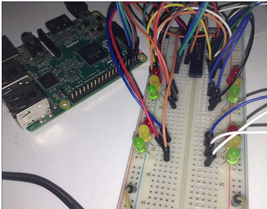
The next step is to build a program for a traffic light controller. The idea is similar as the previous section.
