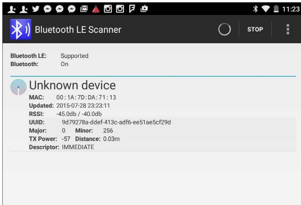
To obtain the details of the Bluetooth device, you can tap the data to see the device information. A sample of the detail information can be seen in the following figure:
