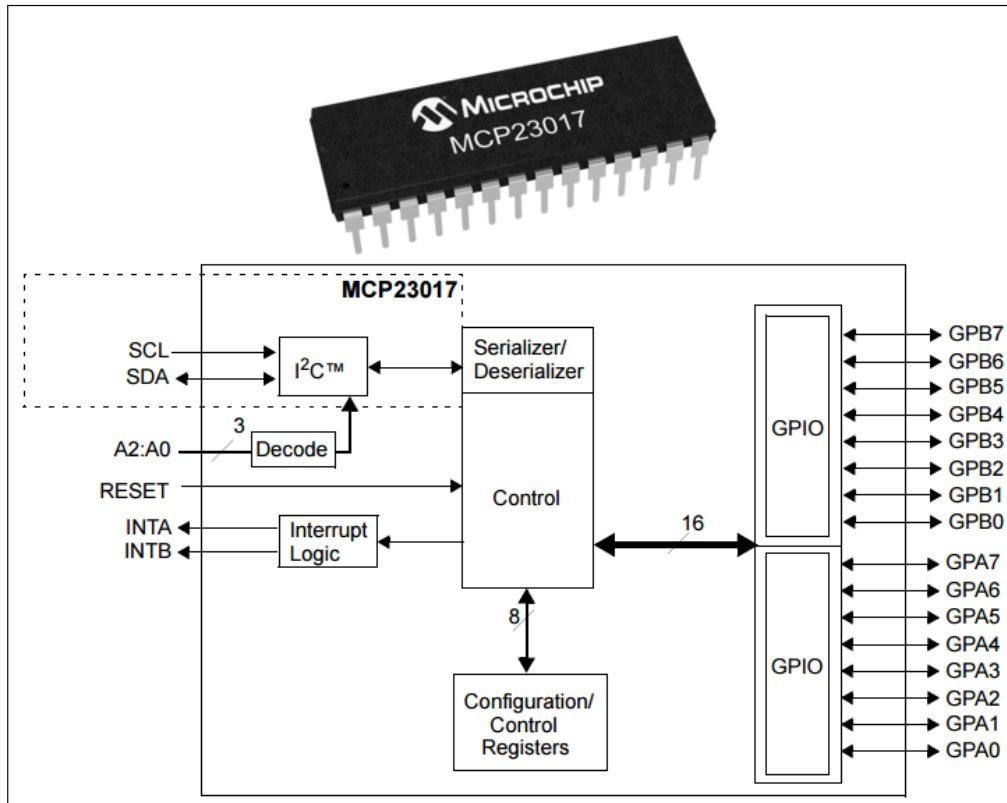
You can control I/O on the MCP23017 via I<sup>2</sup>C on Raspberry Pi. We already learned how to work with I<sup>2</sup>C on Raspberry Pi in *Chapter 3, Make Your Own Digital Clock Display*. To write a program based on I<sup>2</sup>C, we can use the python-smbus module. We are going to use the same approach to access the IC MCP23017.
