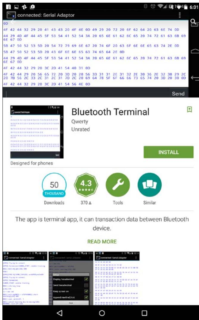
After getting it installed, you can pair HC-06 Bluetooth to Android. By default, the pair key of HC-06 Bluetooth is 1234.
