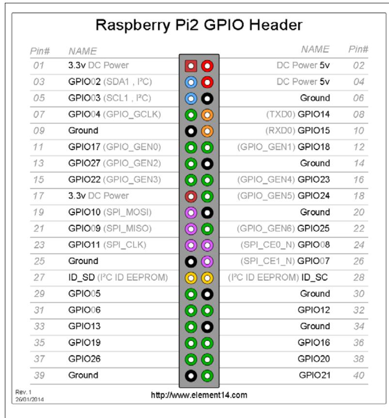
To access Raspberry Pi GPIO, we can use several GPIO libraries. If you are working with Python, Raspbian will have already installed the `RPi.GPIO` library to access Raspberry Pi GPIO. You can read more about `RPi.GPIO` at <https://pypi.python.org/pypi/RPi.GPIO>. You can verify the `RPi.GPIO` library from a Python terminal by importing the `RPi.GPIO` module, as shown in the following screenshot:
