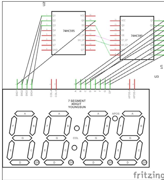
You can also use the 4-digit 7-segment display module with two 74HC595 shift registers easily. For instance, you can get this module on eBay (<http://www.ebay.com/itm/291244187011>) or Amazon (<http://www.amazon.com/Digital-Display-Module-Board-Arduino/dp/B00W9J08I4/>). This module uses a 7-segment common anode.
