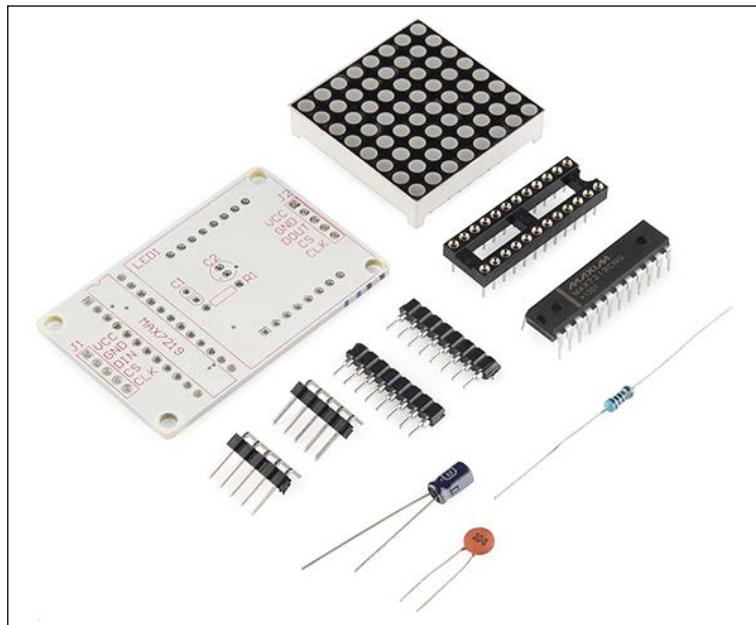
For testing, we use an LED dot matrix module with a 7219 driver. You can buy this module from eBay. The dot matrix display is connected to IC MAX7219 and has the *VCC*, *GND*, *DIN*, *CS*, and *CLK* output pins.
