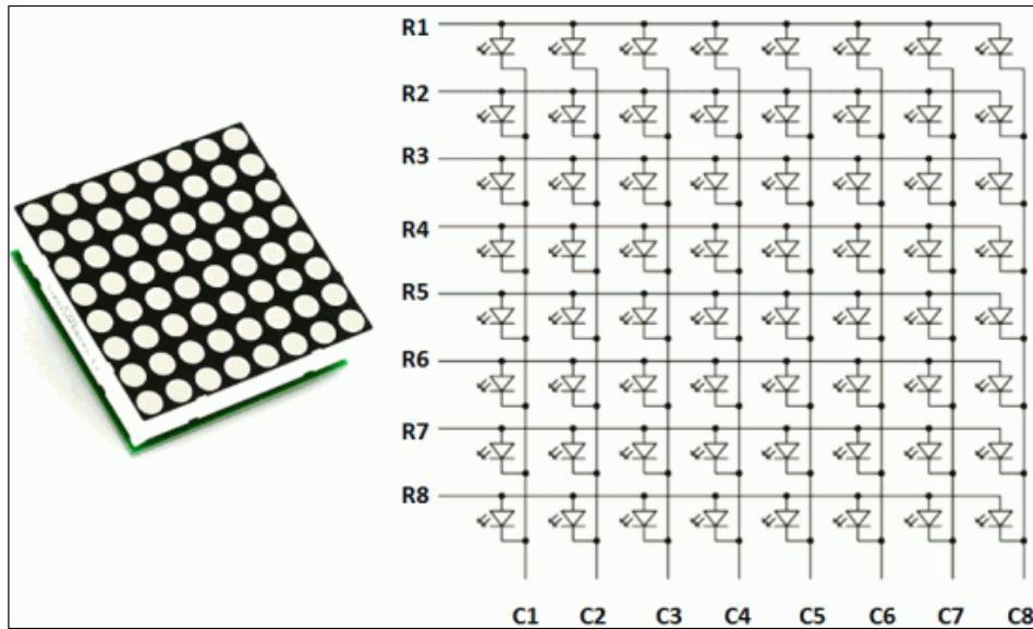
In the preceding figure, if R3 is in 1 logic and C2 is in 0 logic, the LED on line 3 column 3 will be turned on. The characters will be displayed by fast scanning each row and column. For illustration, if we need to display the character A, we can draw the following figure on our dot matrix:
