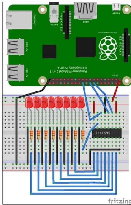
When the output enable (*OE*) input is high, the outputs are in the high-impedance state. Otherwise, (*OE*) input is high. Data in the storage register appears at the output whenever the output enable input (*OE*) is low. A low level on **Master reset (MR)** only affects the shift registers. So in this scenario, we set +3.3 V on the *MR* pin.
