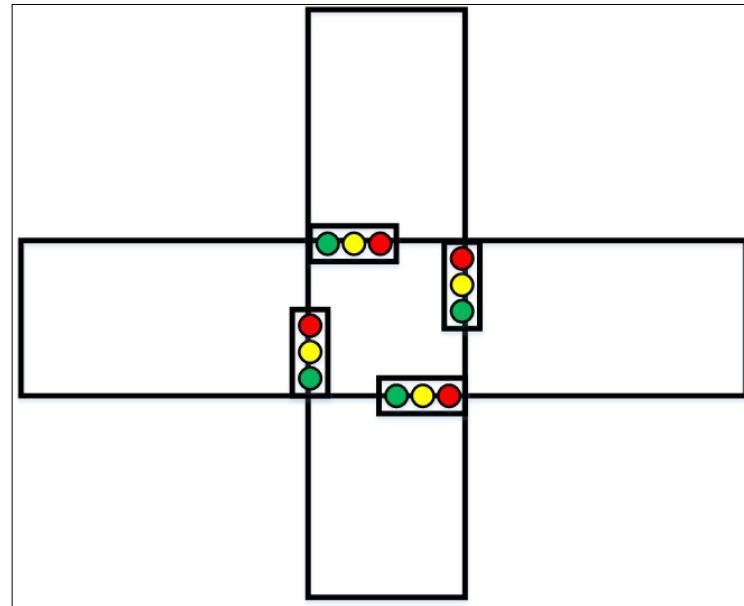
In general, there can be two, three, four or  $n$  road intersections. We know that a traffic light needs three lamps, so to implement  $n$  road intersections, you need at least  $3n$  lamps. You may need walking and *do not work* lamps. Some traffic road intersections can be seen in the following figure:
