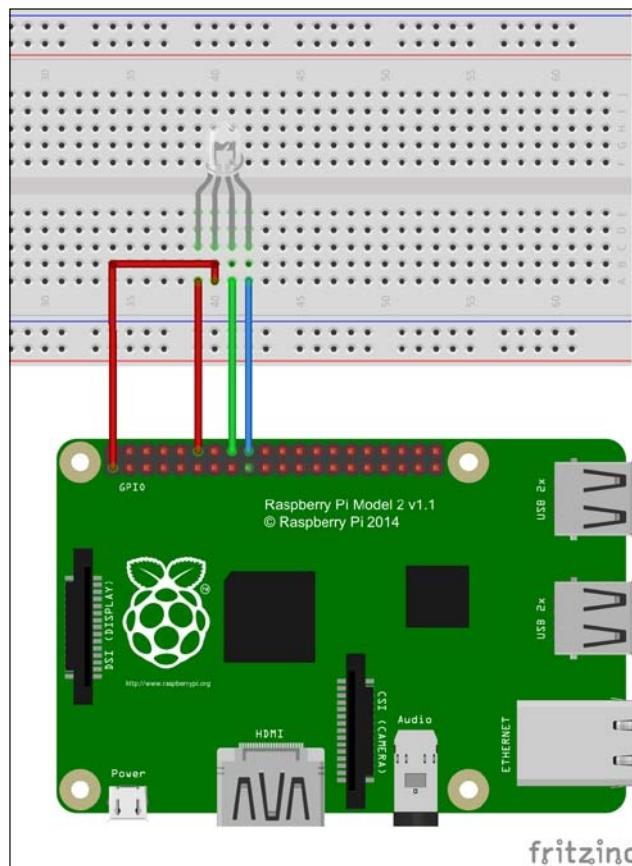
Returning to the Raspberry Pi terminal, you could write a Python program to display color through RGB LED. Let's create a file named `ch01_03.py` and write this script as follows:
