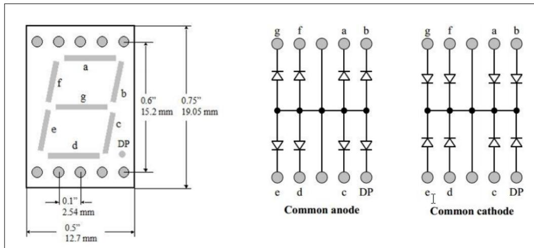
We can show a number on the 7-segment display by combining LED lighting through its pins. For instance, if we want to display the number 7, we should turn on LEDs *a*, *b*, and *c*. To turn an LED on/off, we can use Raspberry Pi GPIO:
