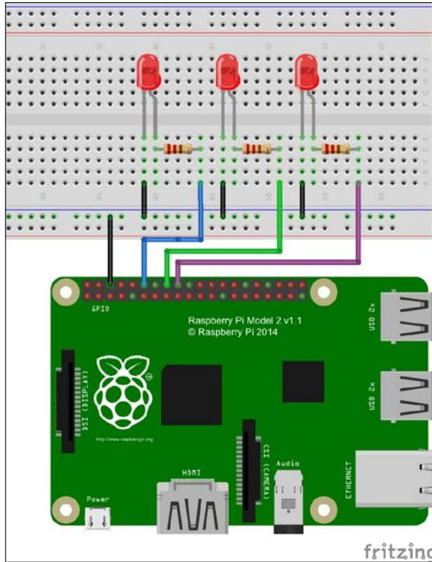
Now you can write a program using WiringPi with Python. The following is the complete Python code for blinking LEDs:
