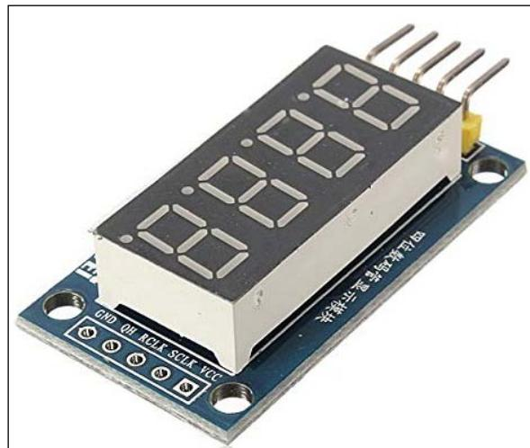
Connect the *DS/ Data*, *STCP/ LATCH*, and *SHCP/ Clock* pins from the first 74HC595 to Raspberry Pi *GPIO25* (wPi 6), *GPIO24* (wPi 5), and *GPIO23* (wPi 4).
