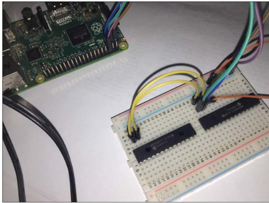
The next is to write a program. You can write a program using I2C as usual. Make sure that each IC MCP23017 already sets its I2C address through  $A_0$ ,  $A_1$ , and  $A_2$  pins.
