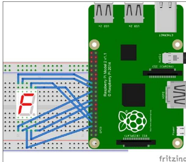
Now we know the hardware wiring, we can write a program to display a number on the 7-segment display using Python. Create a file named `ch02_01.py`. The following is the complete code for the `ch02_01.py` file:
