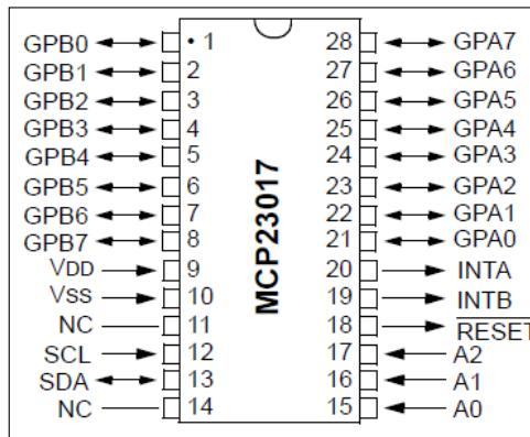
Since the IC MCP23017 has 16-bit I/O pins, you can see the first 8-bit pins located on *GPA0* to *GPA7* and the second 8-bit pins held by *GPB0* to *GPB7*. In this demo, we use only three pins on *GPA0*, *GPA1*, and *GPA2*.
