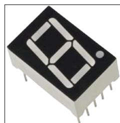
There are two types of LED 7-segment displays, named **common cathode (CC)** and **common anode (CA)**. Each LED has two connecting pins: the **anode** and the **cathode**. A sample LED datasheet can be found at [http://www.kitronik.co.uk/pdf/7\\_segment\\_display\\_datasheet.pdf](http://www.kitronik.co.uk/pdf/7_segment_display_datasheet.pdf).
