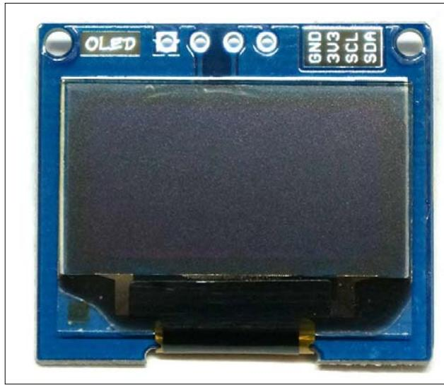
The I2C OLED graphic display has the following pinouts: *GND*, *3V3*, *SCL*, and *SDA*. These pinouts match with your Raspberry Pi I2C.
