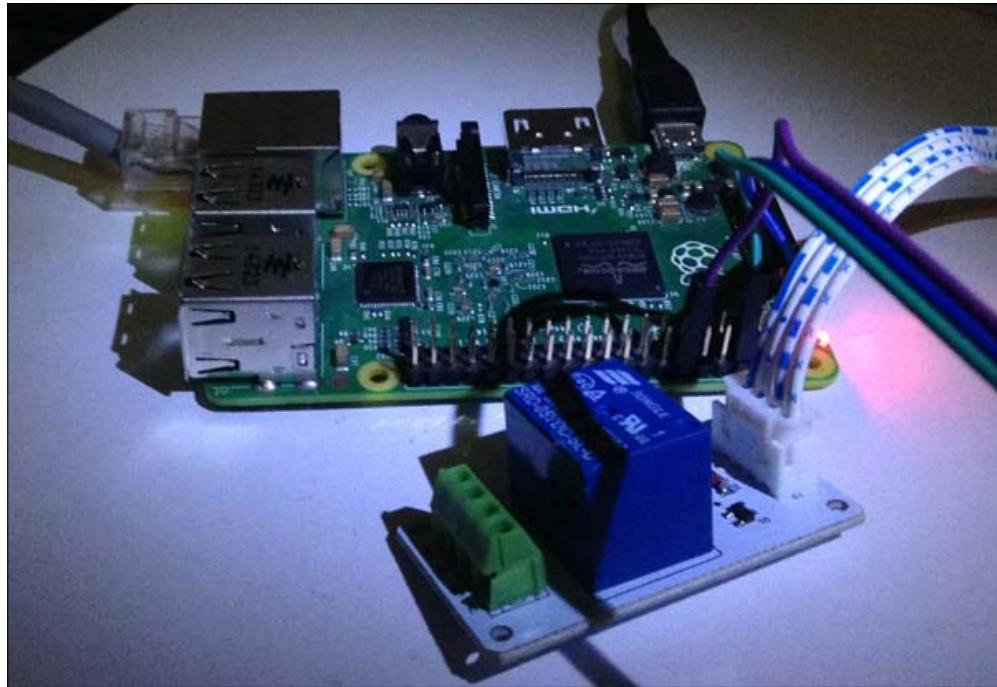
Now we start to write a program. Because we connect our lamp to the *NC* pin, it means we can turn on the lamp by sending a *high* value to the channel relay module. We will develop a simple app for blinking lamps.
