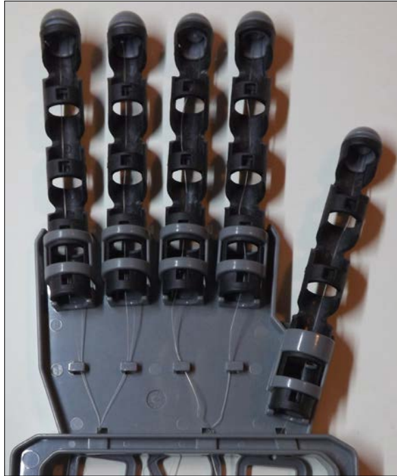
The precision control of servos means they can be used for a variety of applications. For example, controlling simulated hands
