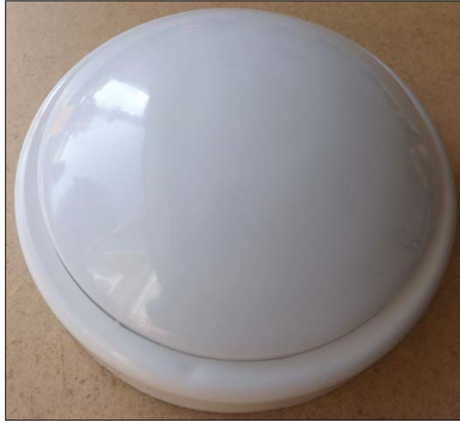
This push nightlight forms the basic chassis of a Rover-Pi robot
