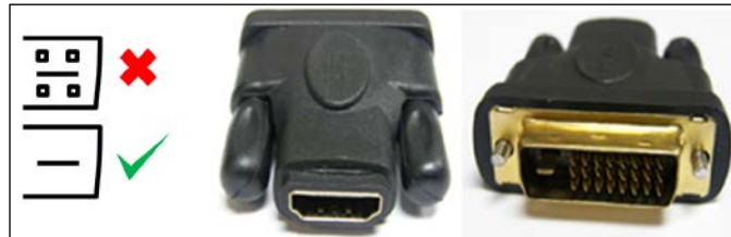
HDMI-to-DVI connection (DVI-D adaptor)
