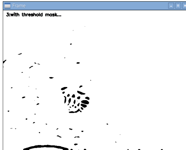
A threshold filter is applied to the delta image, highlighting the largest changes in the image
