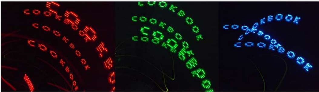
Persistence of vision using RGB LEDs
