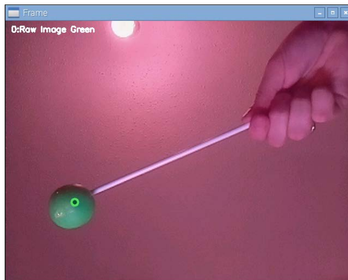
The location of the object is marked with a colored spot as it tracked within the image
