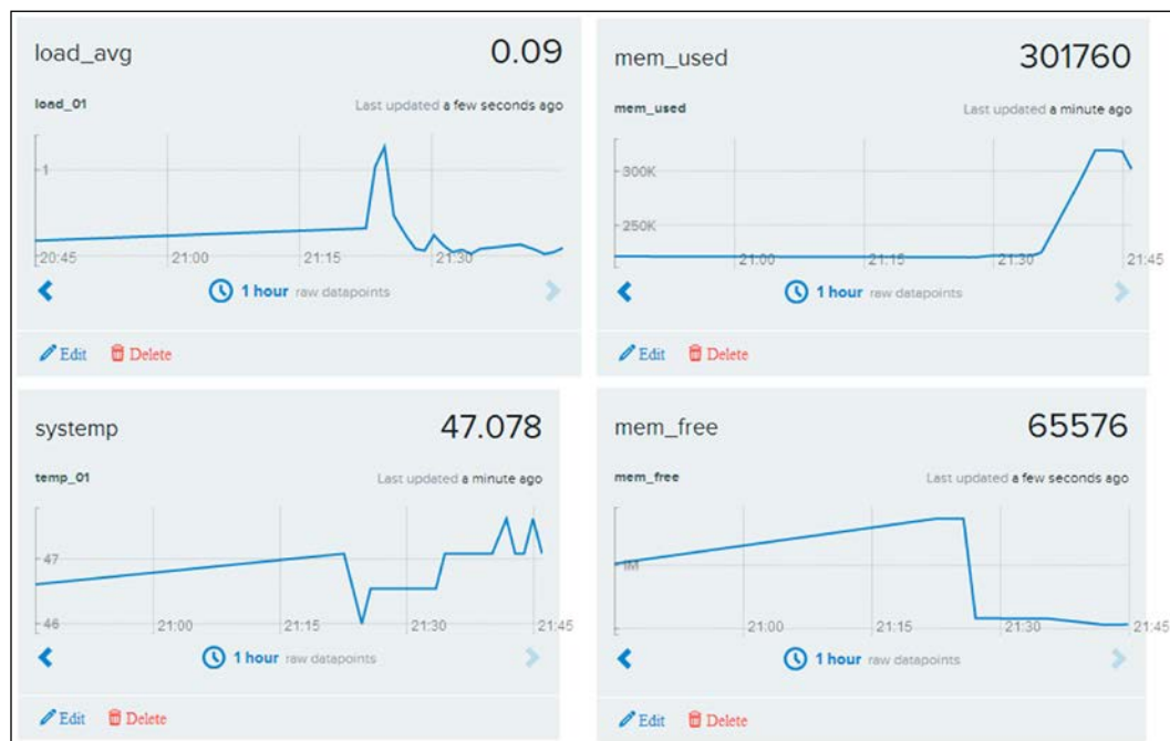
Xively collects and graphs data transferred using REST
