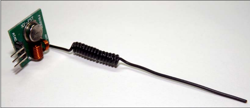
The transmitter range is vastly improved with a simple antenna
