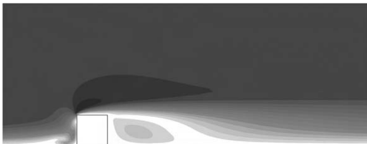
Figure 4.20. Contours of velocity magnitude in the xy symmetry plane.
