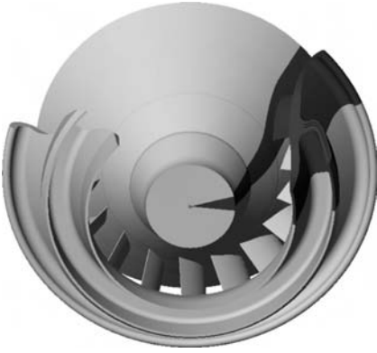
Figure 2.3. The passages through guide vanes of a combustor illustrate periodicity. The geometry is shown in cutaway, with the periodic sector darkened. Figure courtesy of Jorg Schluter.
