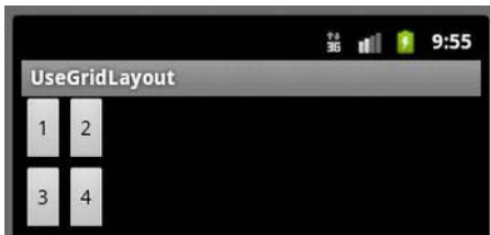
Figure 7-11. The buttons appear small because the default values of gridlayout 's width and height properties are each set to WRAP_CONTENT .
