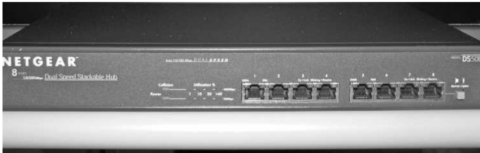
Figure 2-4 A typical hub with indicator lights
