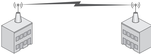
Figure 3-5 A point-to-point wireless topology
