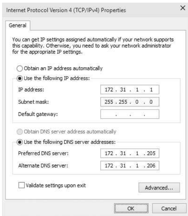
Figure 6-1 A subnet mask based on the address class
