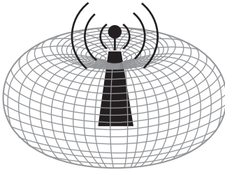
Figure 3-22 The radiation pattern of an omnidirectional antenna
