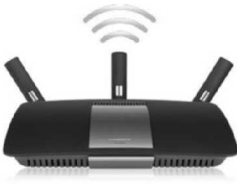
Figure 2-9 A wireless router combines an access point, a switch, and a router
