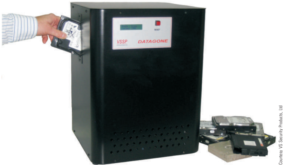
Figure 12-11 Use a degausser to sanitize a magnetic hard drive or tape
