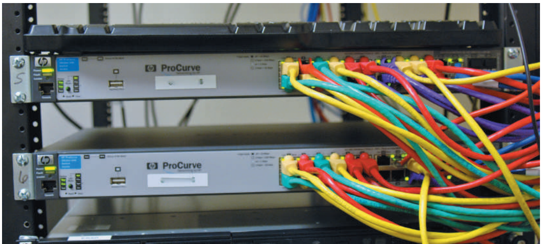
Figure 4-8 Different colors of cables can indicate the general purpose of each cable
