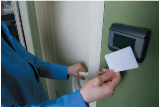
Figure 12-7 A proximity card does not require physical contact with a proximity reader
