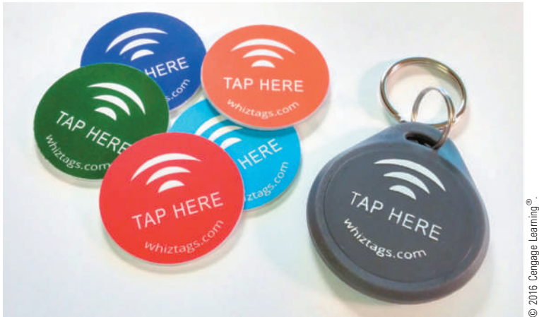
Figure 6-7 These programmable NFC tags have sticky backs for attaching to a flat surface like a wall, desk, or car dashboard
