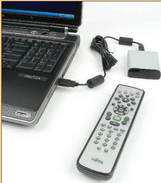
Figure 6-8 This remote control is an infrared device that uses an IR transceiver connected to a notebook by way of a USB port.
