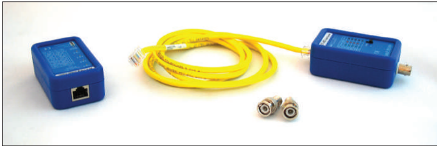
Figure 5-50 Use a cable tester pair to determine the type of cable and/or if the cable is good
