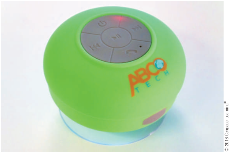
Figure 6-6 The flashing red light indicates this Bluetooth device is in discoverable mode for pairing with a smartphone or MP3 player
