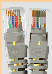
Figure 5-20 Two crossed pairs in a crossover cable are compatible with 10Base-T or 100Base-T Ethernet; four crossed pairs in a crossover cable are compatible with Gigabit Ethernet
