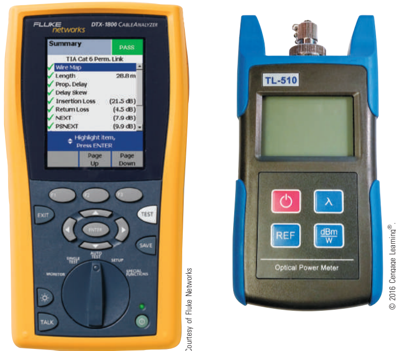
Figure 5-51 On the left, the DTX-1800 device by Fluke Networks is a high-end cable performance tester designed to certify structured cabling. The optical power meter on the right is a more budget-friendly device that measures light power transmitted on a fiber-optic line.
