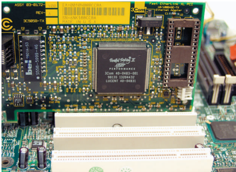
Figure 4-35 An expansion card NIC properly inserted in a PCI expansion slot
