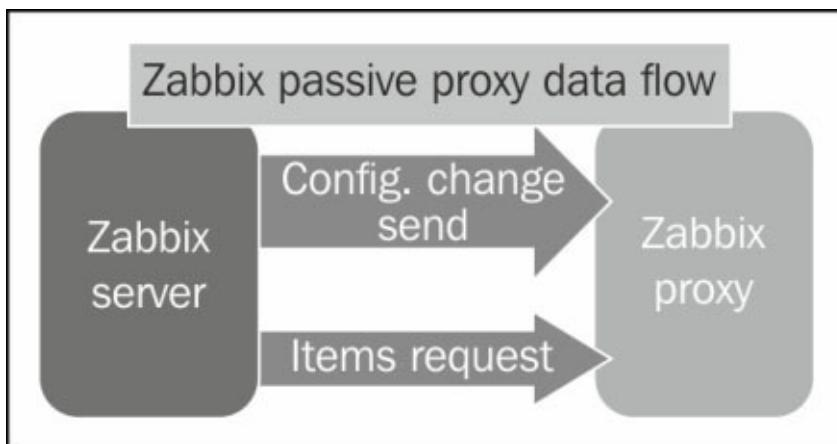
With this configuration, the Zabbix server will contact the proxy periodically to deliver the configuration changes and to request the item values the proxy is holding.
