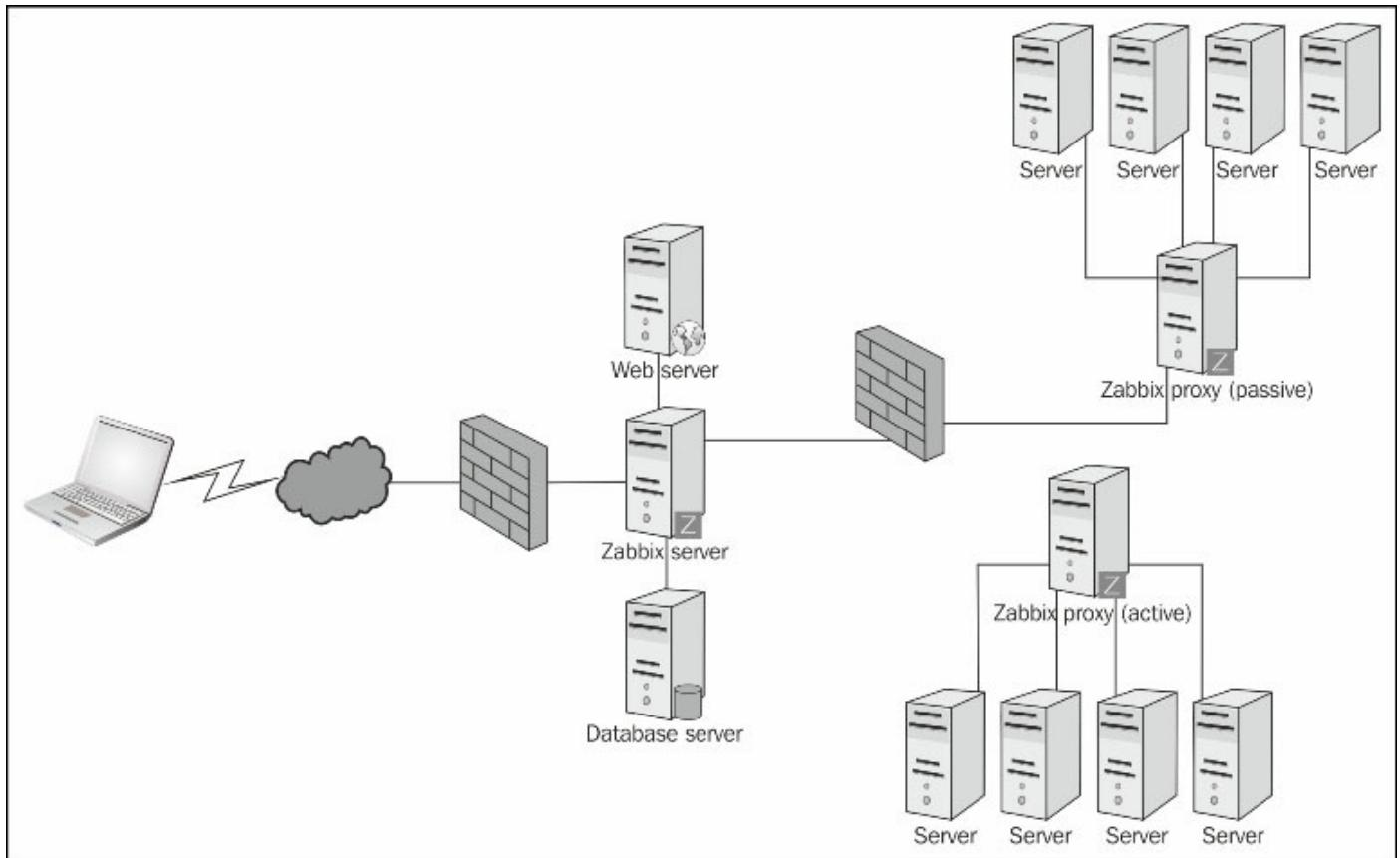
The Zabbix proxy, like a server, is used to collect data from any number of hosts or devices, acquiring all the metrics requested and acting as a proxy. This means that it can retain this data for an arbitrary period of time, relying on a dedicated database to do so. The proxy doesn't have a frontend and is managed directly from the central server.
