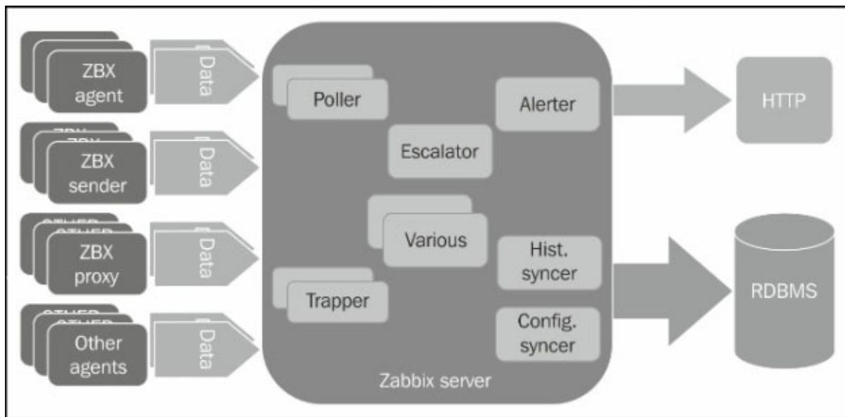
As the diagram displays the data that gets acquired from many different sources in the form of items. At the end of the diagram, you see the GUI, which practically represents the users connected and the database that is the place where all the values are stored.
