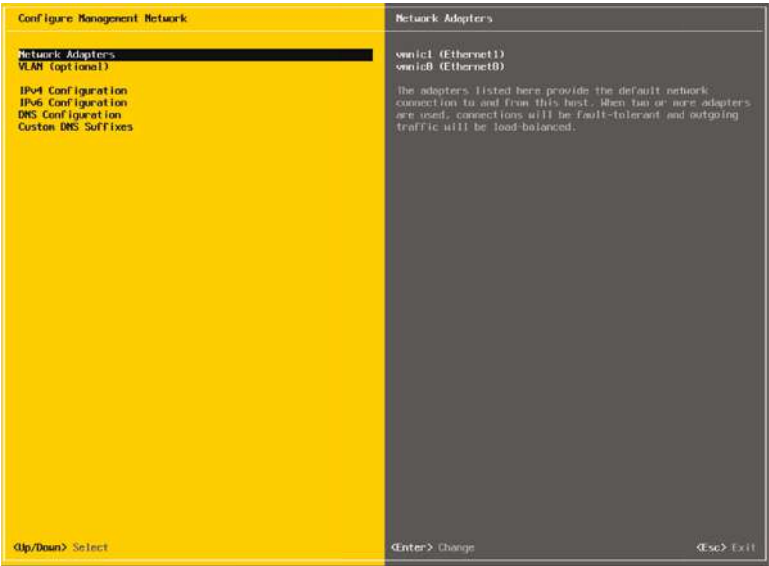
FIGURE 5.11 From the Configure Management Network menu, users can modify assigned network adapters, change the VLAN ID, IP address, DNS Servers, and DNS search configuration.
