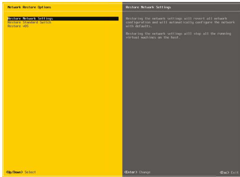
FIGURE 5.13 Use the Network Restore Options screen to manage network connectivity to an ESXi host.
