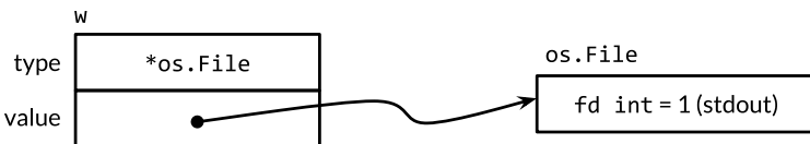
Figure 7.2. An interface value containing an *os.File pointer.
