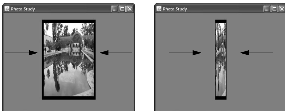
Figure 8.3 Scaling an image along one axis provides the illusion of rotation
