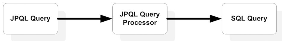
Figure 10.2 Each JPQL query is translated to a SQL query by the JPQL query processor and executed by the database. The query processor is supplied by the JPA provider, most likely the application server vendor.
