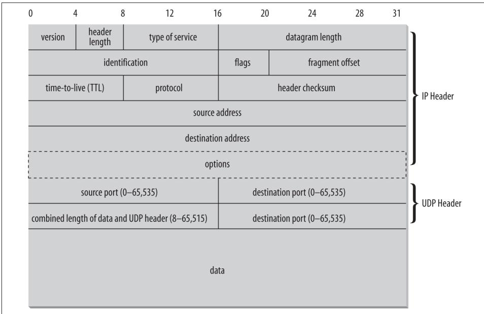
Figure 12-1. The structure of a UDP datagram
