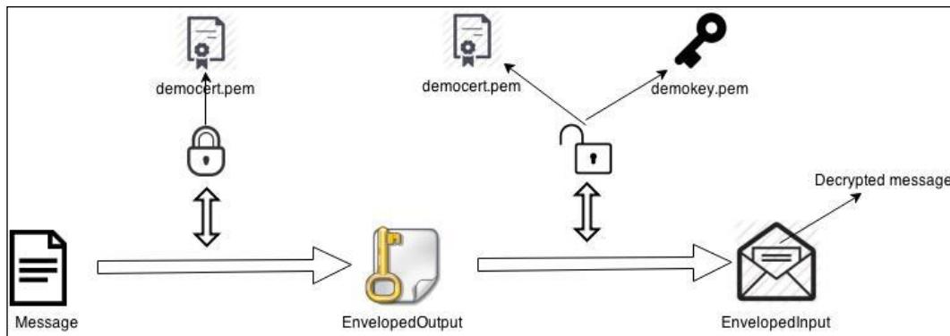
This will be demonstrated in the following code through a unit test. However, before going forward, we want to show that when encrypting messages with S/MIME, headers remain readable but the message body is fully encrypted. So, if we do not have the resources, the information is outdated and cannot be interpreted.
