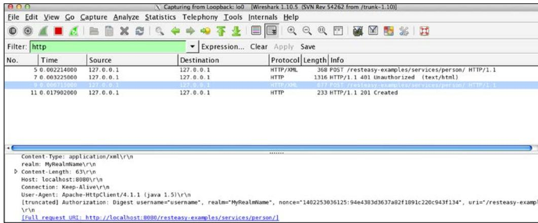
As shown in the screenshot, let's first confirm that all the steps described earlier are performed in this authentication method. Let's keep track using the **No** field in Wireshark:
