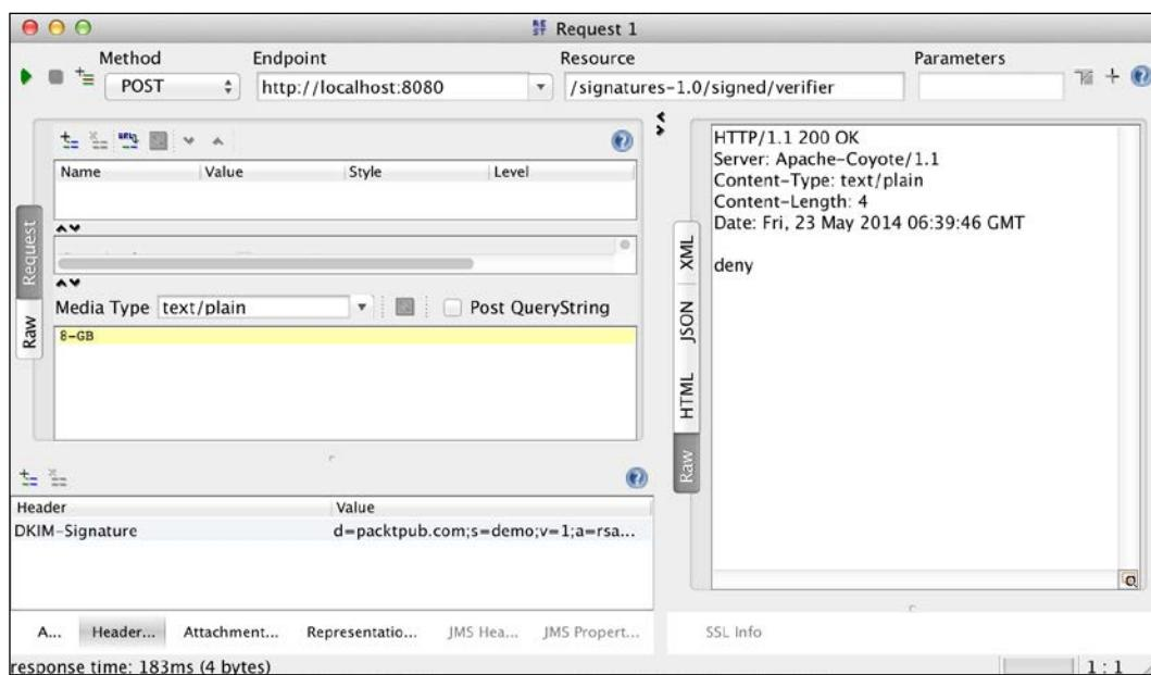
As we can see, the request was successfully processed, but the boss denied the increase of memory. Now, we indicate that digital signatures allow us to validate that the information is not altered once it has been signed. Suppose malicious software intercepted the response, and instead of 8-GB, it delivered the value 12-GB. Let's make this request in SoapUI following the theory of digital signatures. This request should not be valid; however, we must check:
