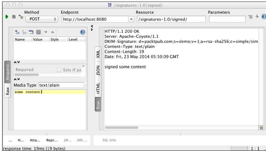
As you can see in the response, we obtain the `DKIM-Signature` header used to sign the message. The full content of this header is as follows:
