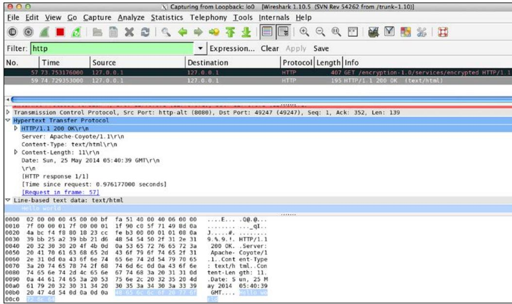
As we can see, the traffic analyzer shows how all the information is traveling straight and how easily it is interpreted. Now, let's enable HTTPS on JBoss to show how the whole message is encrypted.
