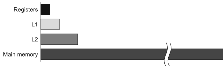
Figure 6.3 Relative access times for registers, processor caches, and main memory
