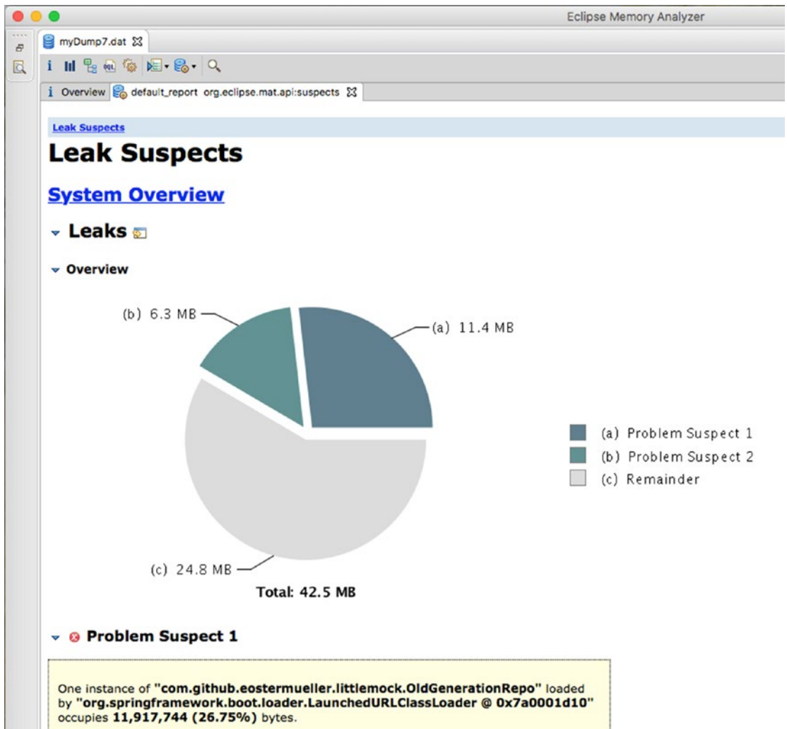
Figure 12-10. Eclipse MAT Leak Suspects looking at a heapDump from littleMock. In perhaps a third to a half of the heap dumps I have seen, this screen points reasonably close to the the leaky instances and/or the object containing them.
