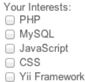
Figure 9.2: The checkboxList() method creates multiple checkboxes from an array.
