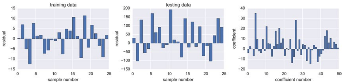
Figure 15-2. The residual between the Ridge regularized regression model and the training data (left), the model and the test data (middle), and the values of the coefficients for the 50 features (right)
