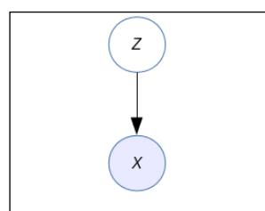
This represents the probability distribution  $P(X, Z)$  where, this time, the  $Z$  node is white to indicate that it is hidden or latent. If we marginalize out the variable  $Z$  from this model to obtain the distribution on  $X$  we will obtain exactly the previous formula. Also note that, in this model,  $X$  has a multivariate Gaussian distribution.
