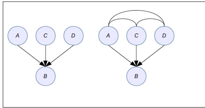
2. Then the graph is transformed into an undirected graph where each arrow is replaced by a simple edge. The effect of the first two operations is that each variable (a node in the graph) and its parent are now in the same clique—that is, a subgraph where the nodes are all connected.
