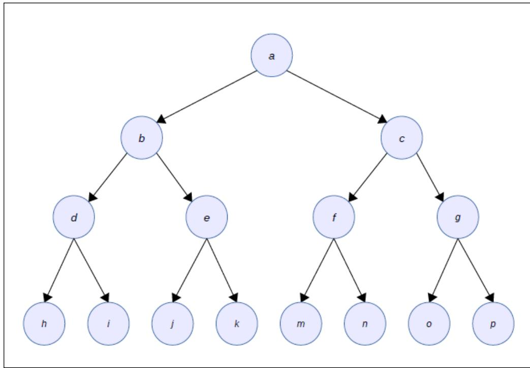
In this model, the clusters of nodes generated by the junction tree algorithm will always be made up of two nodes only: the child and its parent. So this model keeps the complexity of the junction tree algorithm low and allows for fast inference.
