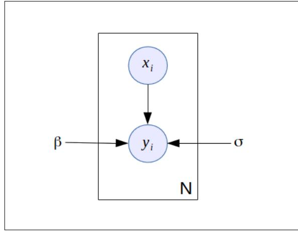
In this graph, it is clearly stated that each  $y_i$  is dependent on one  $x_i$ . It is also clear that the parameters  $\theta = \{\beta, \sigma\}$  are all shared as they are outside the plate.
