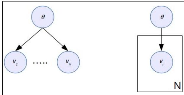
And it's about time we introduced a new notation term for graphical models: **the plate notation**. The left figure is our usual representation in which we only represent the first and the last of the  $v_i$  nodes, to make the figure simpler. This can sometimes be a bit confusing and in many cases ambiguous or cumbersome when one has too many nodes. The right side of the figure represents exactly the same graph where the box means that the node(s) inside are repeated  $N$  times.
